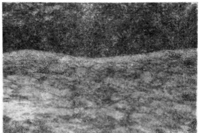
Fig. 3d. Brass to Mild Steel  $\times 75$  (magnification)
