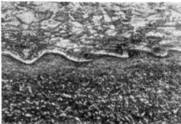
Fig. 3a. Copper to Brass  $\times 75$  (magnification)
