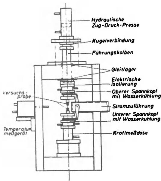
Fig. 2. Press-welding equipment (Schematic).
