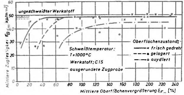
Fig. 7. Relationship between the tensile strength and the degrees of upset for different initial states.
