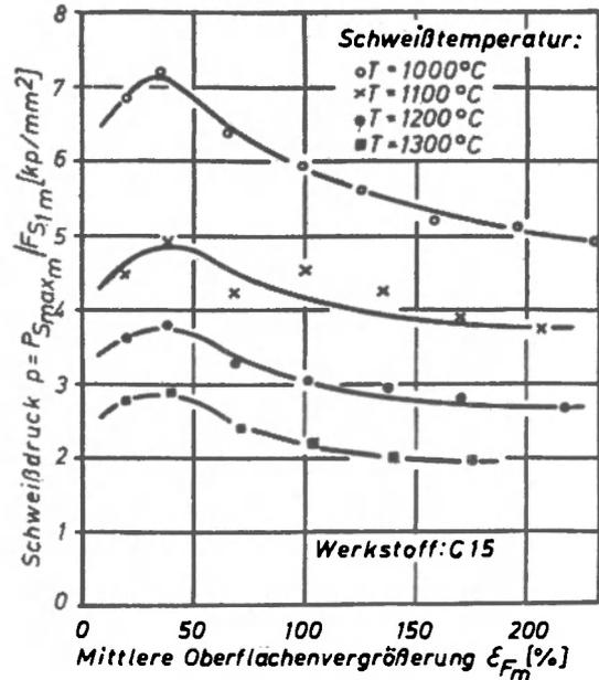
Fig. 12. Relationship between the welding pressure and the degrees of upset for different temperatures.
