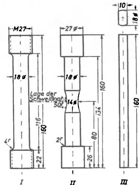
Fig. 5. Test pieces for the testing of raw material.
