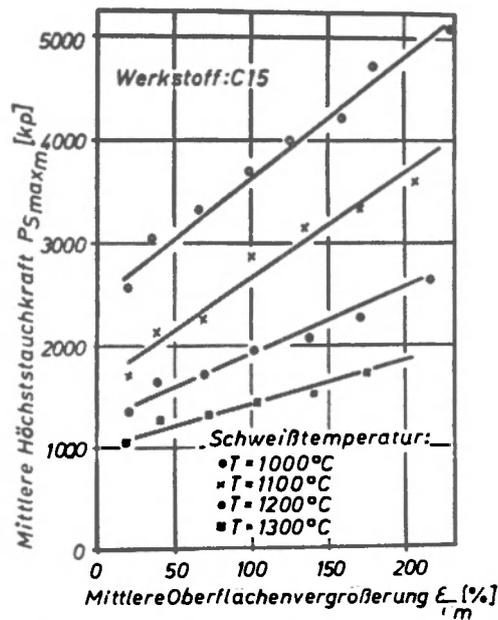
Fig. 13. Relationship between the maximum compression load and the upsetting for different welding temperatures.
