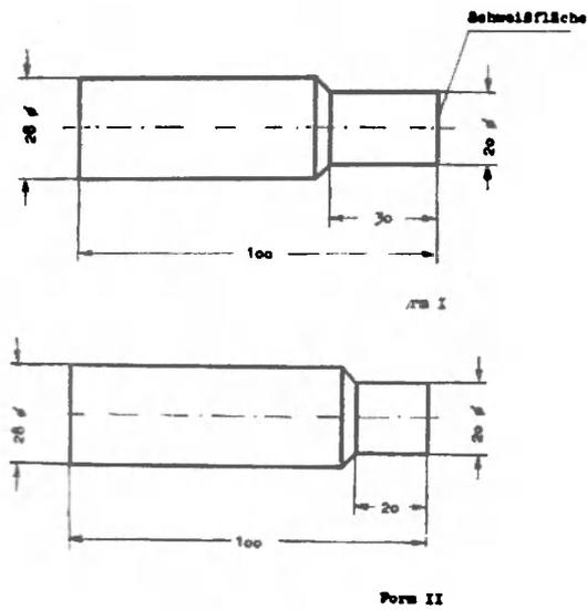
Fig. 1. Test pieces for welding.
