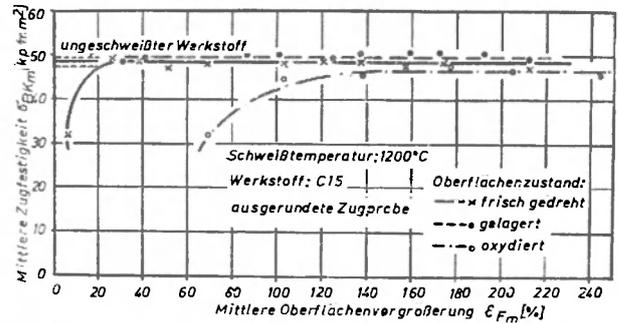
Fig. 8. Relationship between the tensile strength and the degrees of upset for different initial states.
