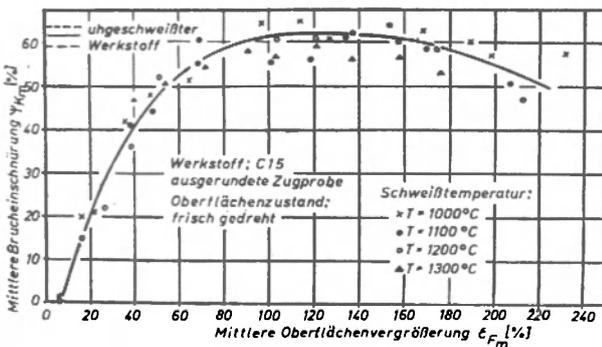
Fig. 11. Reduction in area of cross section at the fracture in relationship with the degrees of upset for different welding temperatures.
