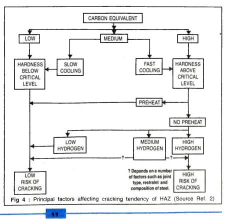
there is risk of cracking; except in thick section, HAZ cracking is rarely experienced with CE values below 0.39%. At high levels of CE, say around 0.48%, there is high risk of cracking even at slower cooling rates. However, appropriate preheating of the parent metal and/or lower levels of hydrogen in the weld metal can eliminate this problem.
