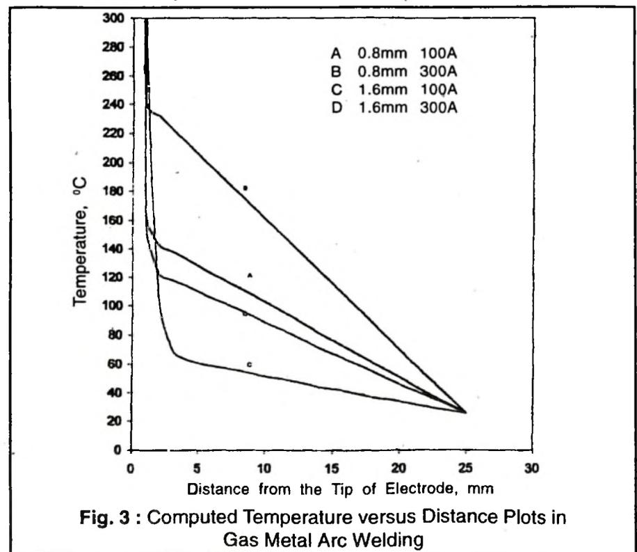
Fig. 3 : Computed Temperature versus Distance Plots in Gas Metal Arc Welding
