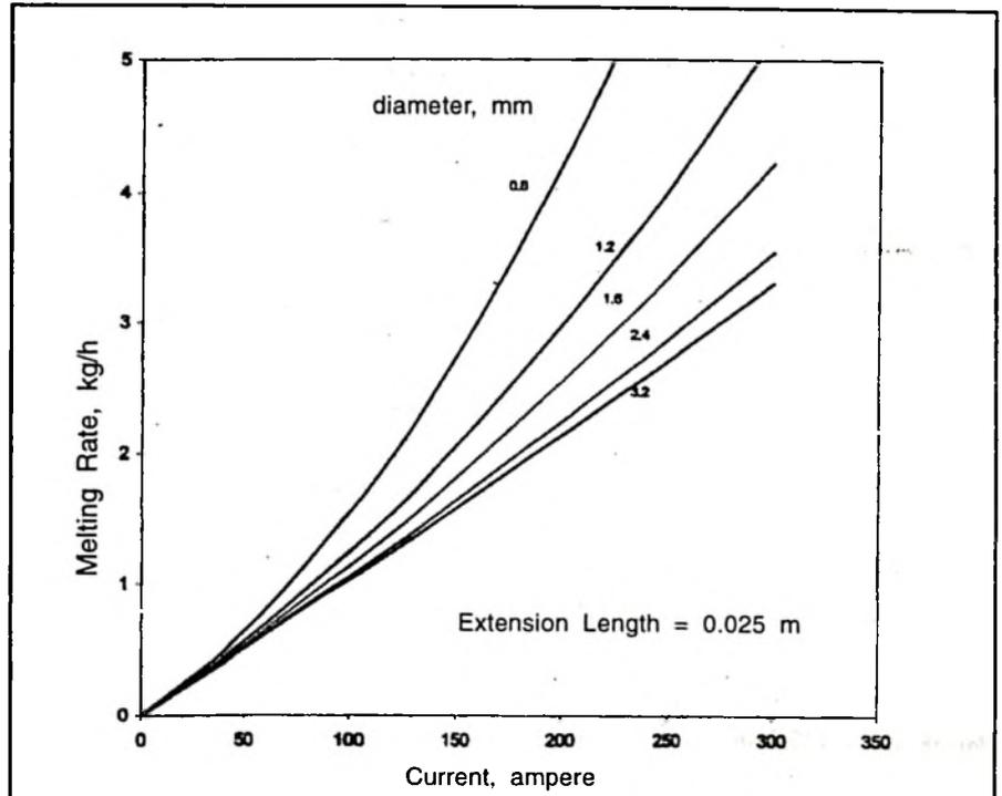
Fig. 1 : Melting Rate versus Current Plots for Arc Welding Processes using Consumable Electrode.
