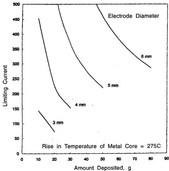
Fig. 5 : Limiting Current versus Weight Deposited Plots for Shielded Metal Arc Welding
