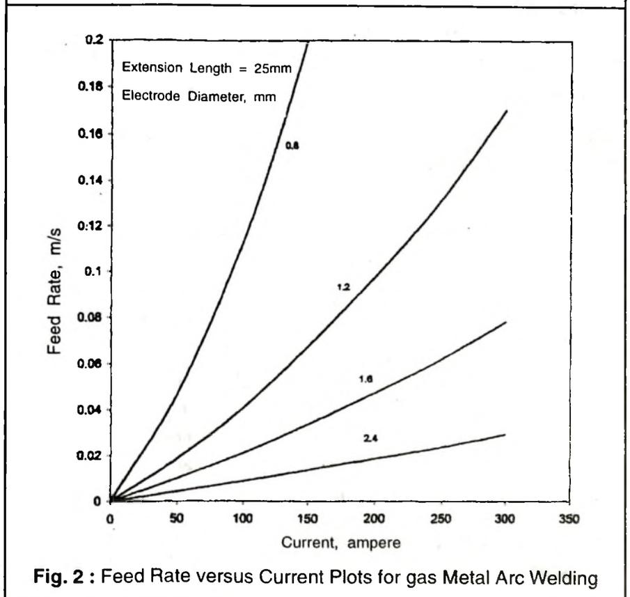
Fig. 2 : Feed Rate versus Current Plots for gas Metal Arc Welding
