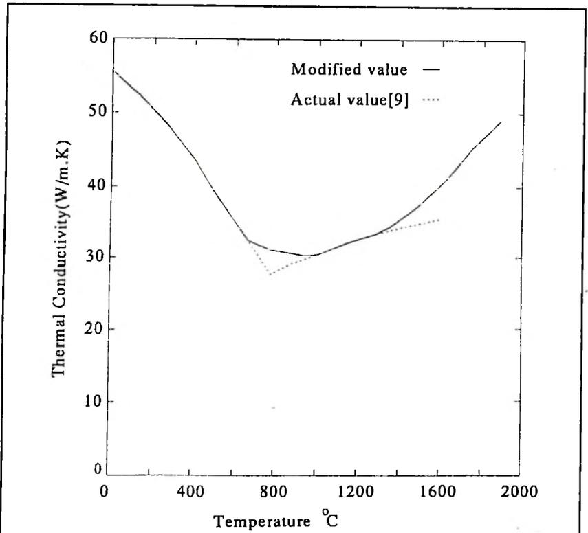
Fig. 1 : Thermal Conductivity of mild steel St 37
