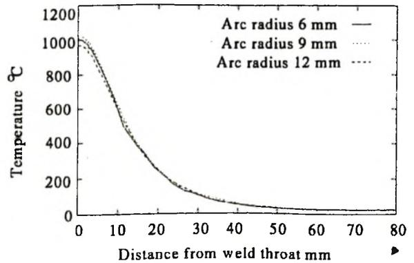
Fig. 10 : Transverse temperature distribution at mid section 7.5 s after passing arc
