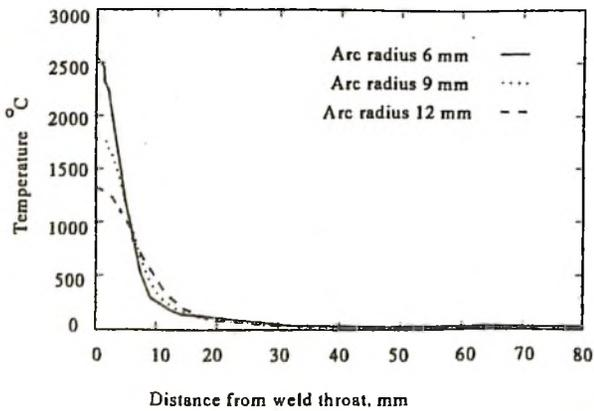
Fig. 9 : Transverse temperature distribution at mid section during passing arc
