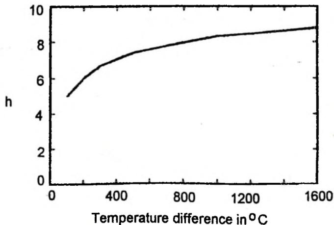
Fig. 3 : Convective heat transfer coefficient [9]
