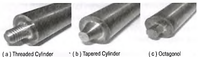
Fig. 1 (a, b, & c) : Different types of tool pin profile
