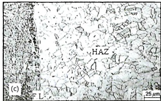
Figure 7 : Typical microstructure of HAZ adjacent to fusion line observed in SMA weld deposit prepared by using (a) Conventional groove (b) Narrow groove with 14mm weld width and (c) Narrow groove with 11mm weld width.
