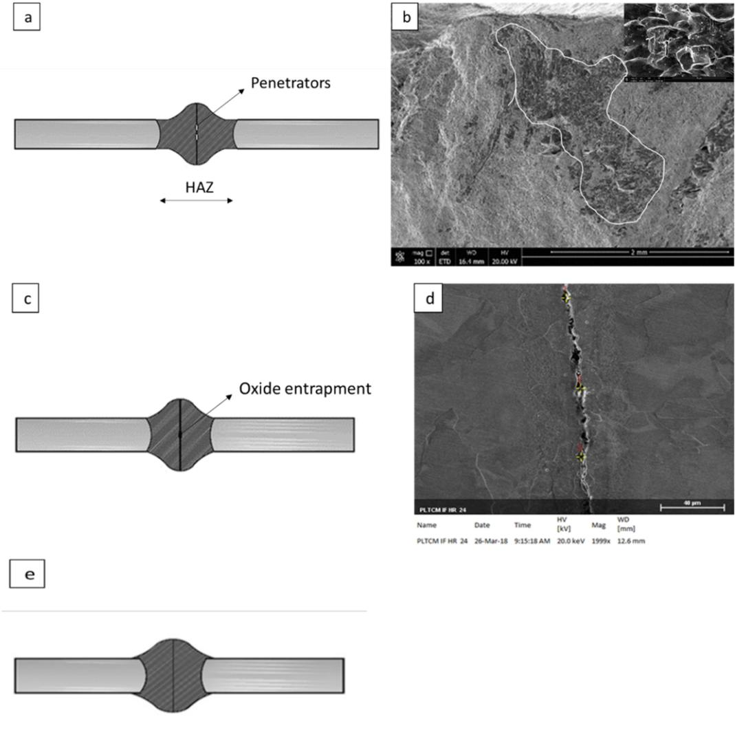
Fig. 4 : Schematic of flash butt weld defects and corresponding SEM images.
