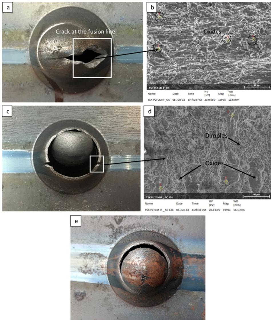
Fig. 3 : Steel A failure analysis (a, b) Parameter 1, (c, d) Parameter 2, and e) Parameter 3
