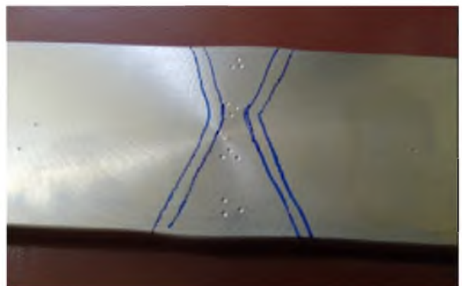
Hardness, HV10 (Weld Cross Section) Photo
