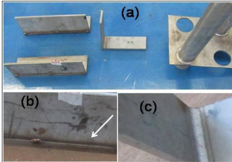
Fig. 3 : Welded test coupons, comprising all types (a), the fillet root (b) with an arrow indicating an incidental gap, and the face of the fillet weld (c).
