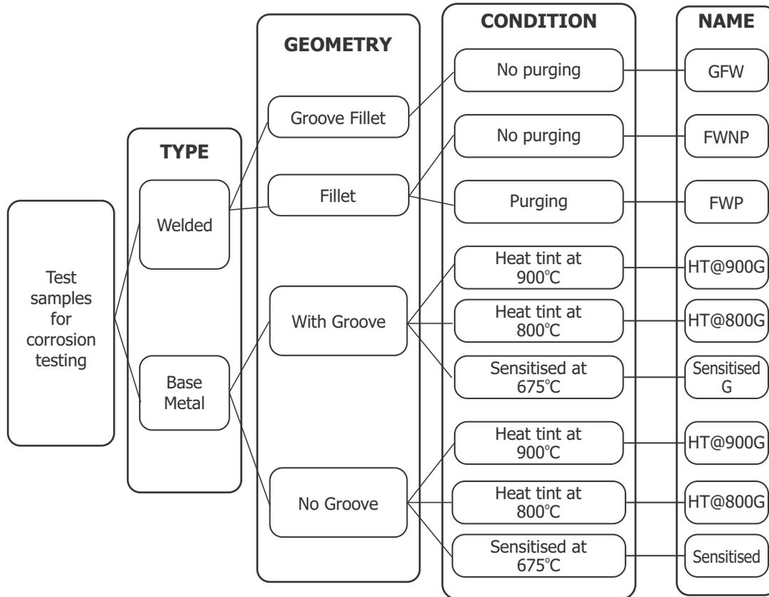
Fig. 1 : Samples plan for corrosion test
