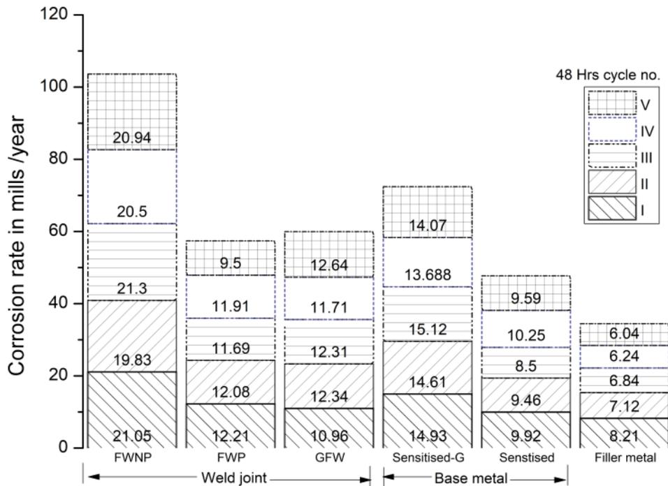
Fig. 8 : Corrosion Rate Comparison among Base Material, Weld Joint, and Un-diluted Filler Metal
