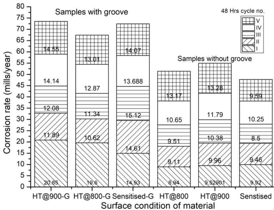
Fig. 7 : Comparison of corrosion rate for base material
