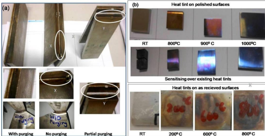
Fig. 4 : Heat-tinted areas (a) on the adjoining surfaces of the root side in fillet weld joints, where no purging or partial purging was employed during welding, and (b) produced on the base metal with both polished and as-received surfaces.
