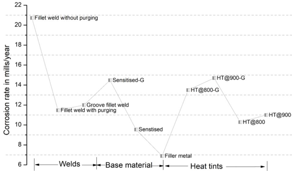
Fig. 6 : Average corrosion rate of all the samples after corrosion tests
