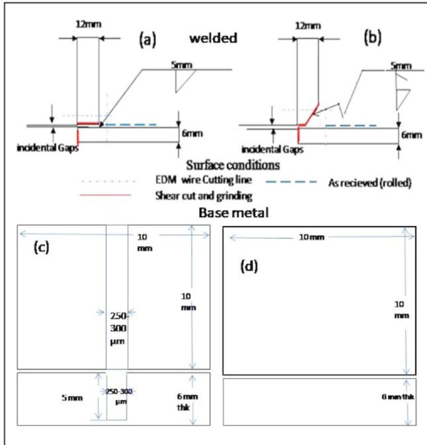
Fig. 2 : Schematics of specimens designated for corrosion testing, including weld joints with fillet (a), groove fillet (b), and base metal both with (c) and without groove (d).
