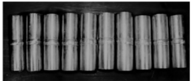
Fig. 4 : Welding of SS304HCu by GTAW process [49]
