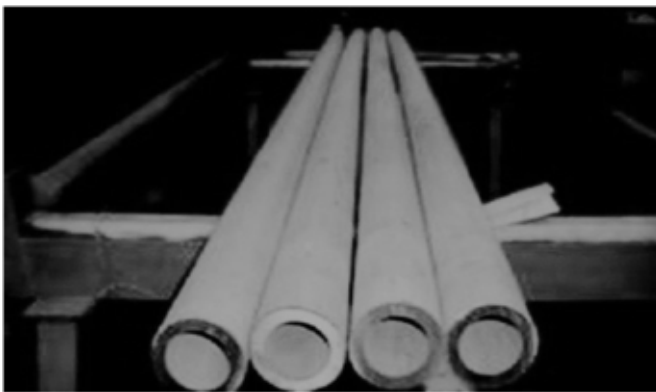
Fig. 3 : Indigenously manufactured Boiler tube of SS304HCu, length 6-7m [49]
