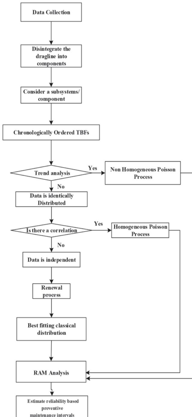
Fig.1 Procedure for analysis of the failure of repairable systems
