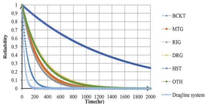
Fig.4 The reliability plots of each subsystem of the dragline
