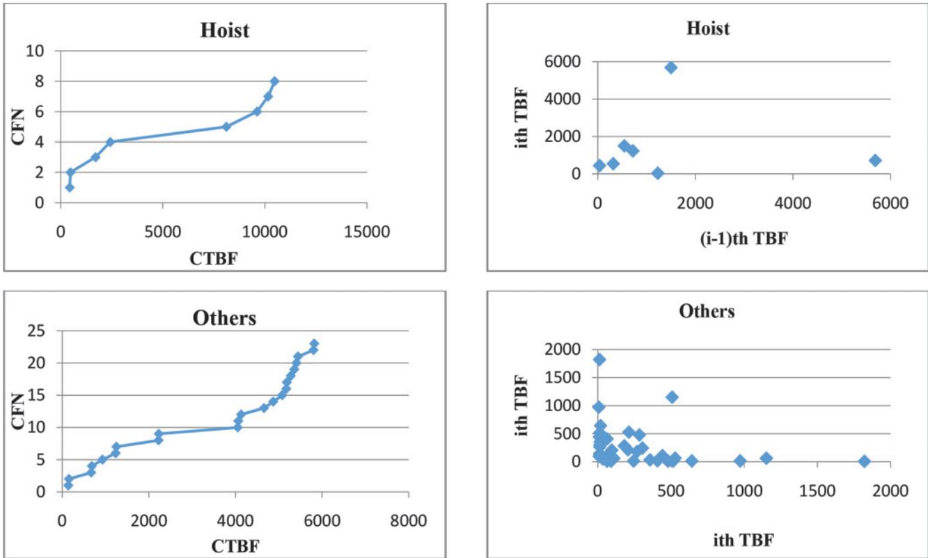
Fig.2 Trend and correlation tests diagram for TBF data of dragline
