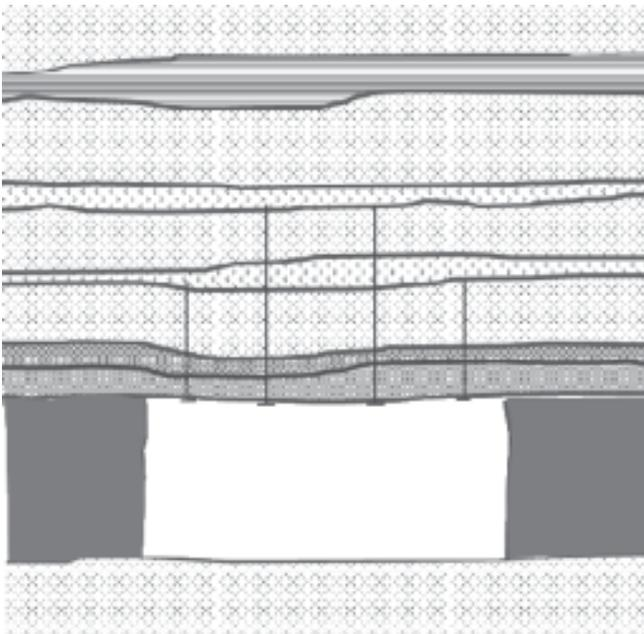
Fig.1 Rock bolt support system in an underground mine opening
