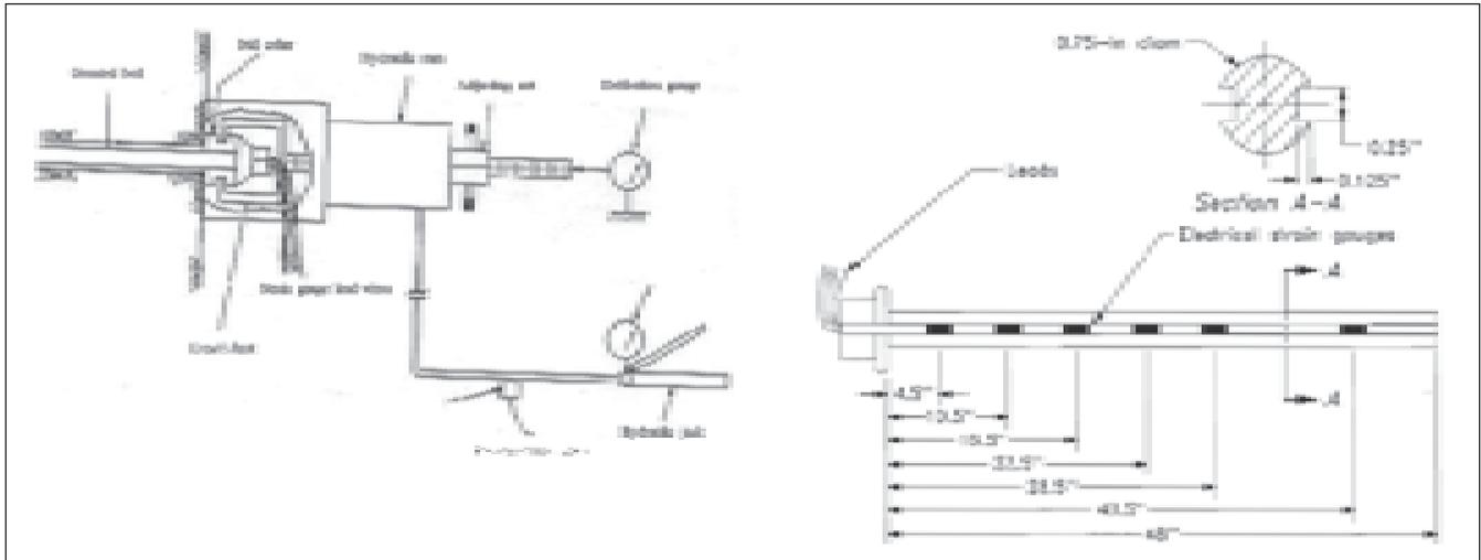
Fig.7a Pull-test arrangement and strain gauged bolt used by Signer (1990)
