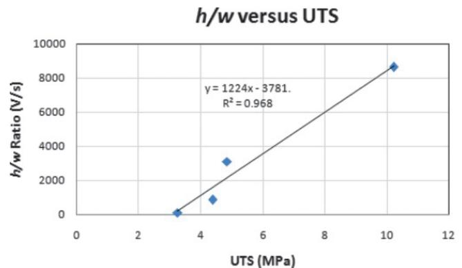
Fig.8: Plot of  $h/w$  vs UTS
