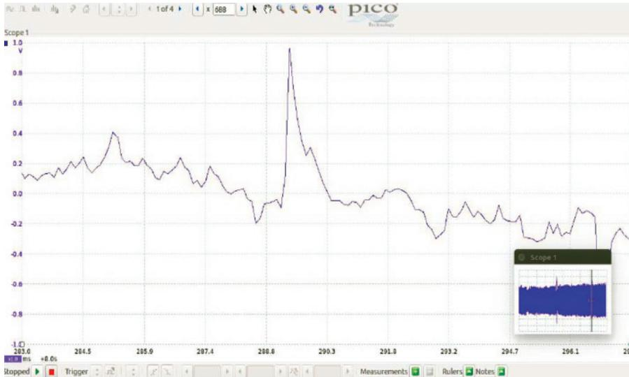
Fig.5: Coarse-grained shaly sandstone voltage vs time graph
