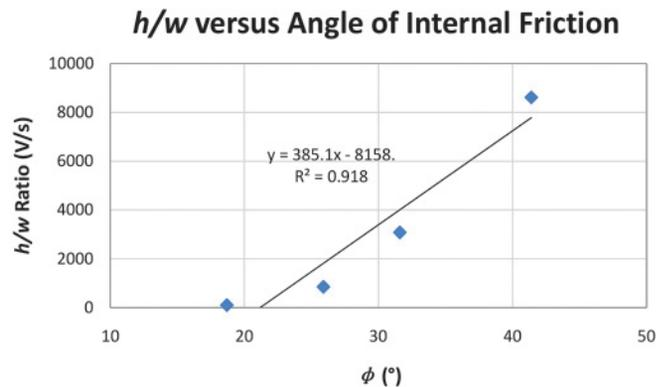
Fig.11: Plot of h/w vs angle of internal friction.
