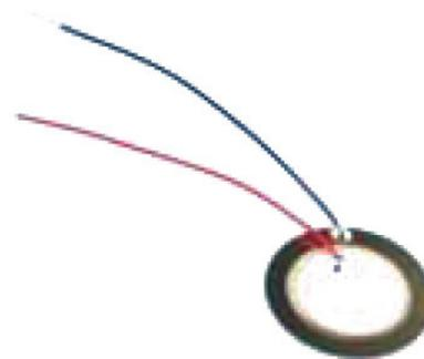
Fig.2: Piezoelectric sensor
