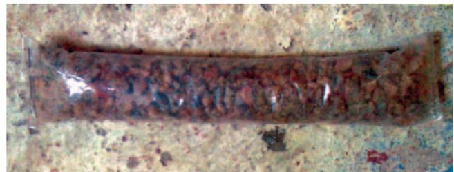
Fig.7 Cartridged packing of crushed angular stones used for ‘decking’
