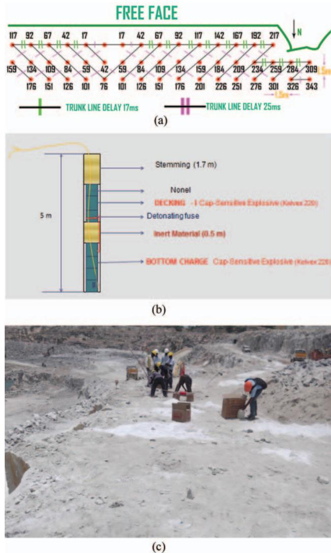
Fig.4 (a) Initiation pattern (b) Modified charging geometry with 'decking' (c) Charging of holes in the site
