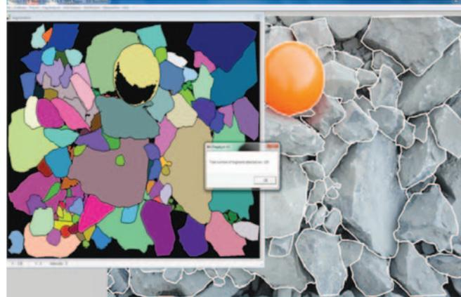
Fig.1 Fragmentation analysis using image analysis software
