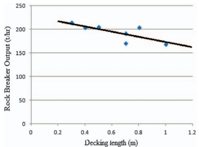
Fig.9 Graph representing the relation between deck lengths and rock breaker performance
