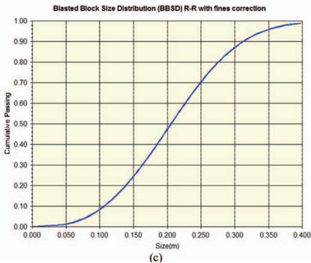
Fig.5.0 (a) Presence of ‘drop’ and coarser fragmentation after the blast (b) Muck pile produced by blasting (c) Fragmentation analysis curve
