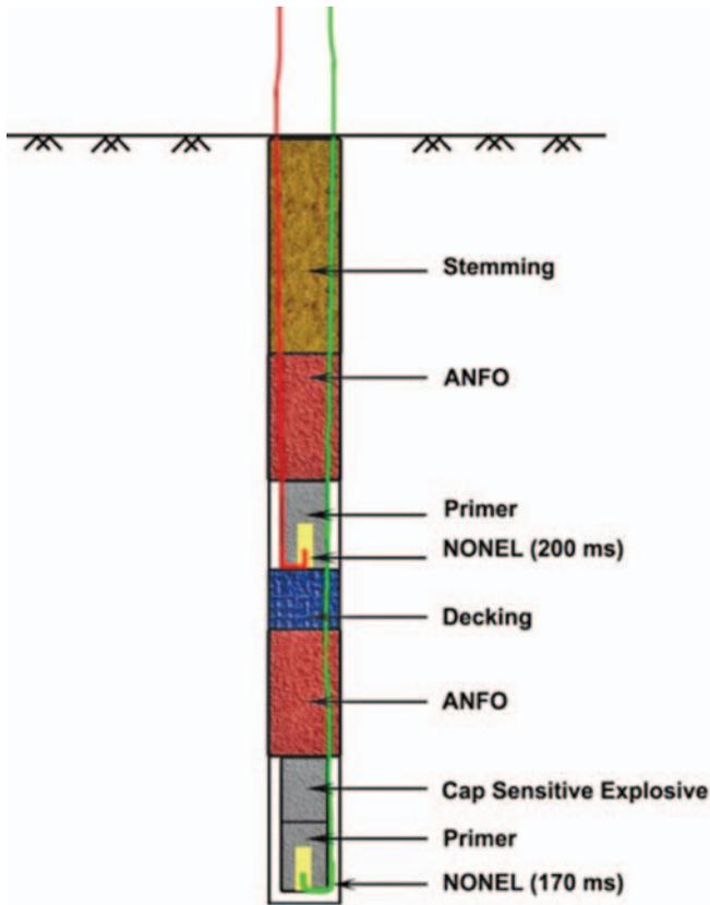
Fig.2 Typical decking practices in the quarry blasting
