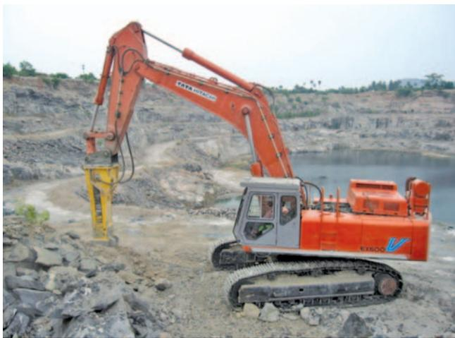
Fig.8 Rock breaker working with blasted muckpile
