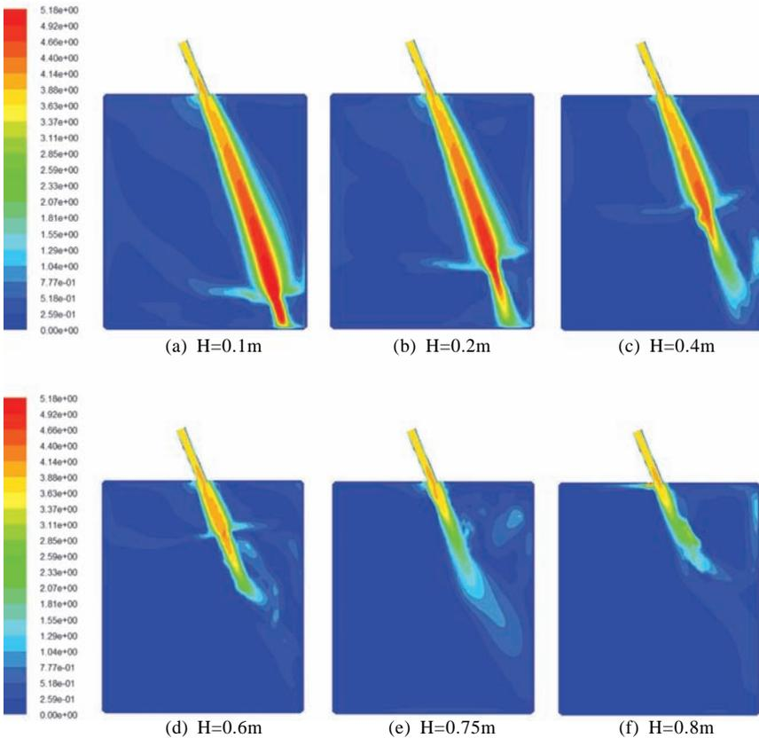
Fig.10 Velocity contours of tangent plane of oil flow
