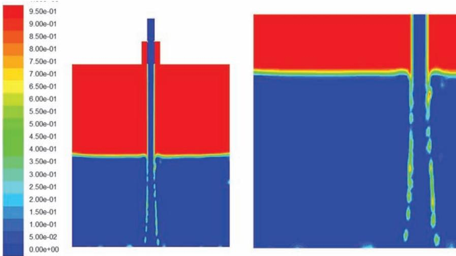
Fig.6 contours of oil and gas volume fraction of the tangent plane of oil flow
