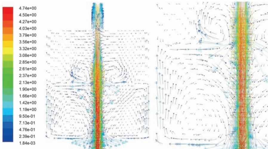
Fig.5 Velocity vectors of oil and gas volume fraction of the tangent plane of oil flow
