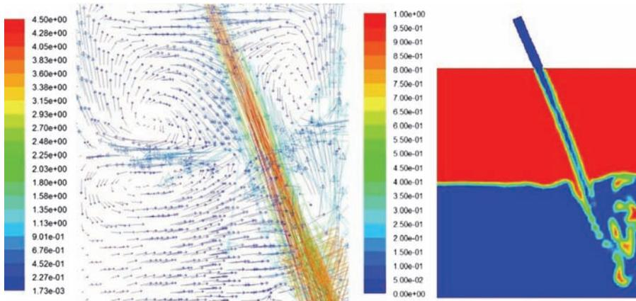
Fig.12 Velocity vectors and contours of oil and gas volume fraction of the tangent plane of oil flow
