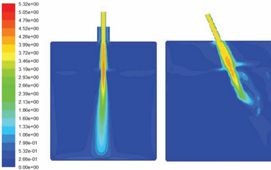
Fig.11 Comparison of velocity contours by two refuelling ways when H=0.6m
