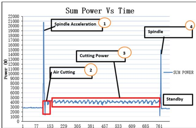
Fig.4: Power profile in slotting
