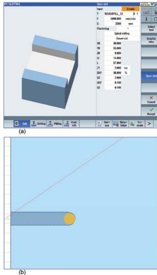
Fig.3: (a) Shopmill interface for slot process (b) Trochoidal toolpath
