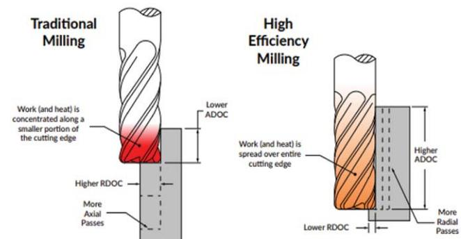
Fig.1: Traditional milling and high efficiency milling [8]
