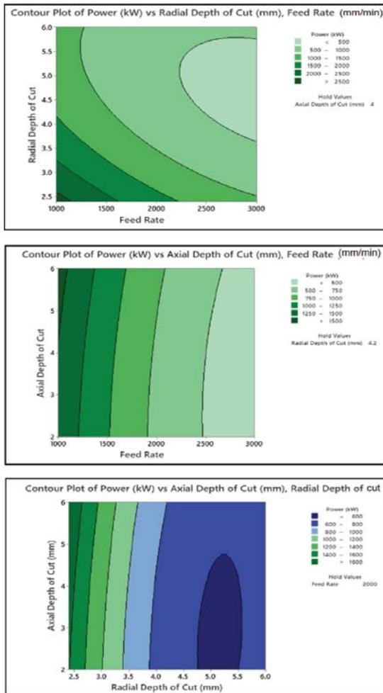
Fig.7: Contour graph of power consumption
