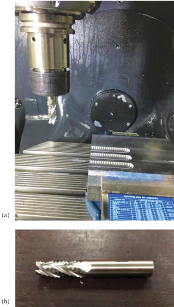
Fig.2: (a) Experimental setup, and (b) Rough flat end mill cutter
