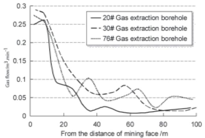
Fig.5 Curves of gas flow change
