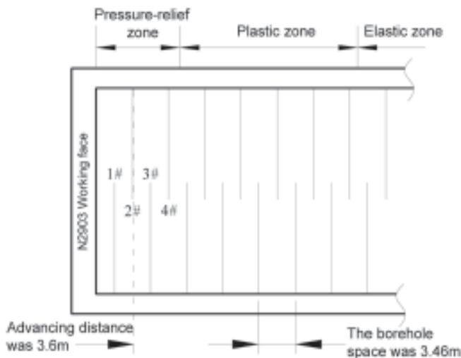
Fig.7 The borehole layout at the mining face
