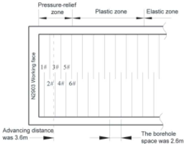
Fig.6 The borehole layout at the mining face
