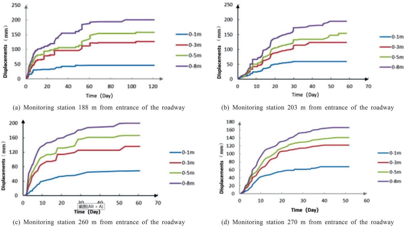
Fig.14 Curves of roof deformation at different locations of the roadway under test
