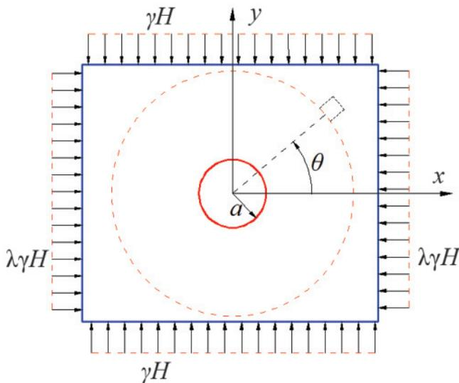
Fig.1 Mechanical model of a circular hole
