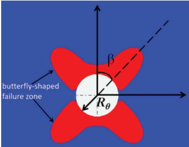
Fig.2 Schematic characterisation of main dimensions of plastic zone in the rock surrounding a roadway
