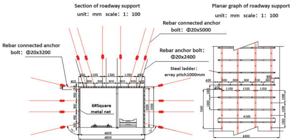
Fig.12 Schematic diagram of flat section in the scheme of combined support with long anchor bolts
