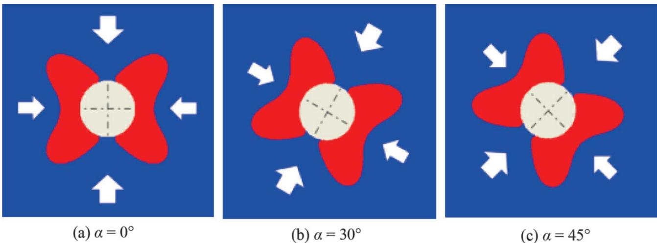
Fig.3 Relationship between shape of butterfly-shaped failure zone and the direction of the principal stress
