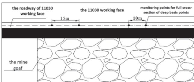
Fig.13 Location of monitoring stations for displacement of deep basis points
