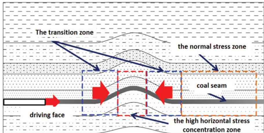
Fig.8 Schematic diagram showing characteristics of the stress environment around the fold
