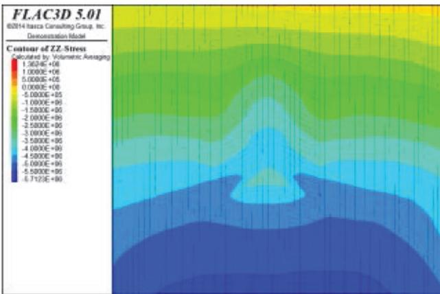
Fig.7 Cloud picture of vertical stress
