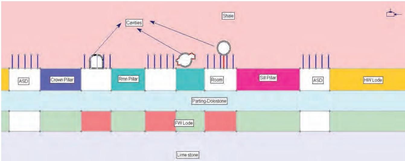
Fig.4 Model geometry of HW lode mining [4]
