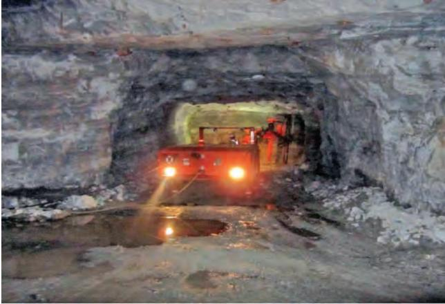
Fig.9 Drilling by extra low profile drill jumbo in development face of FW lode
