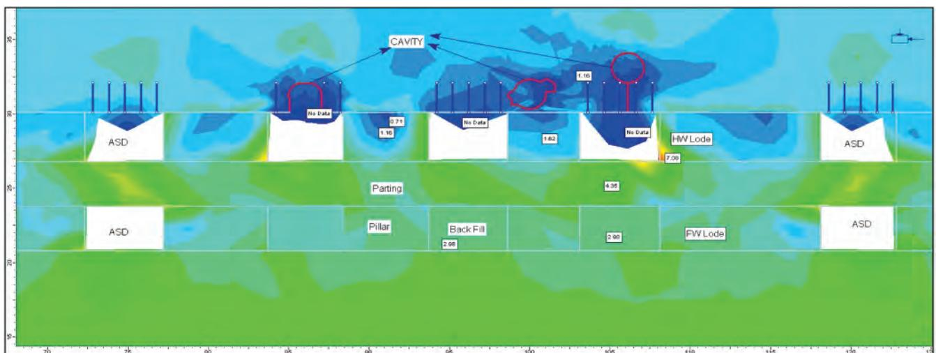
Fig.5 Mining induced stresses around excavations [4]
