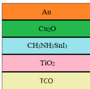
Fig. 1: Structure of the Simulated model of \text{CH}_3\text{NH}_3\text{SnI}_3 PSC
