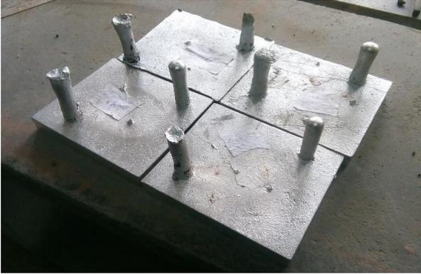
**Figure 4.** Prepared A356-Hematite composite with copper chills.
