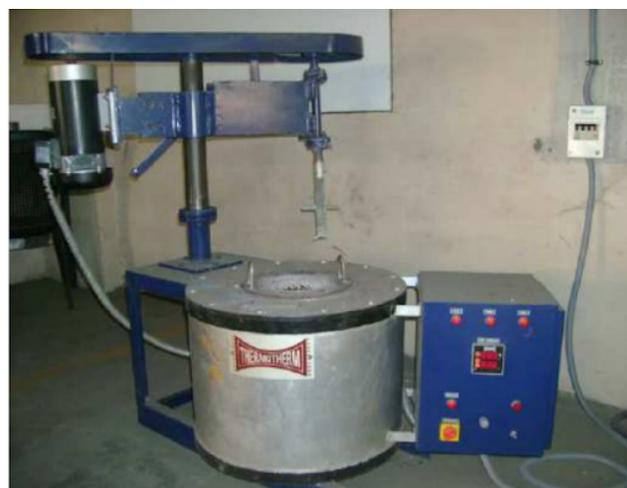
**Figure 2.** Electric Furnace.
