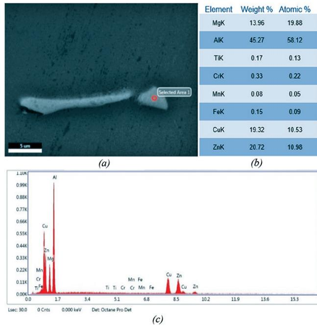
Figure 9: Edx analysis of Al 7175 base alloy
