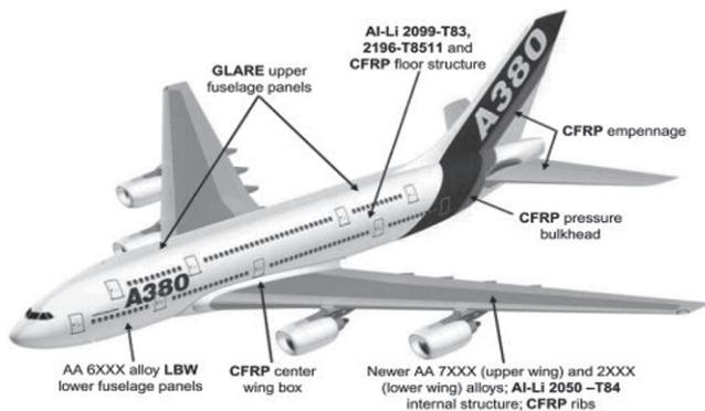
Figure 1: Advanced material used for structural areas of the airbus A380<sup>3</sup>
