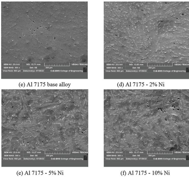
Figure 8: SEM analysis of heat-treated alloy at 300X-200µm
