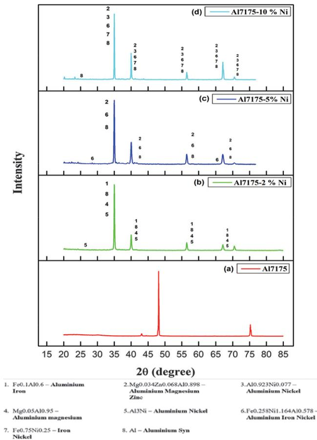
Figure 6: X-Ray diffraction (XRD) analysis of heat-treated aluminium alloy (a) 0% Ni (b) 2% Ni (C) 5% Ni (d) 10%Ni
