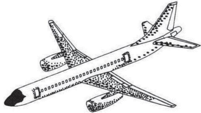
Figure 2: Impact distribution on aeroplane. Source: Adapted from<sup>8</sup>.
