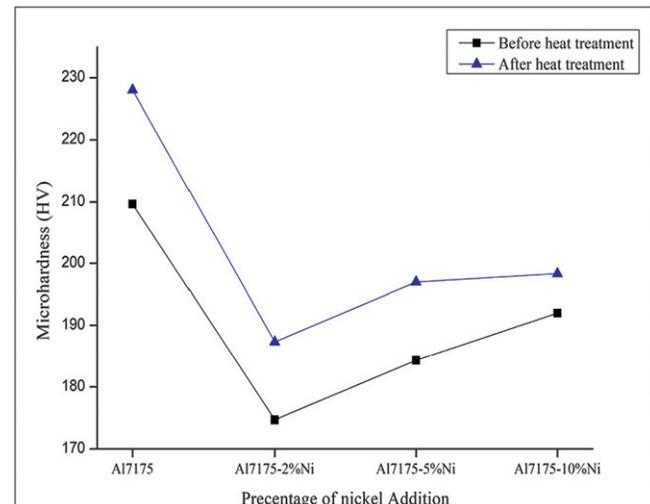
**Figure 3: Variation in the values of hardness with increase in percentage of nickel**
