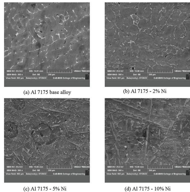
Figure 7: SEM analysis of non- heat-treated alloy at 300X -200µm
