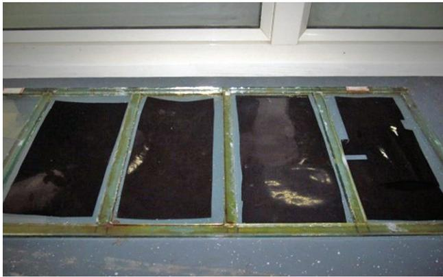
Figure 1: Fabrication mold used for nano CuO-PVA composite films
