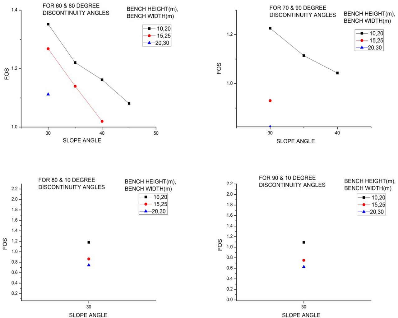
**Figure 18.** Influence of slope angle on FOS for different discontinuity angles and different bench height and bench width combination.
