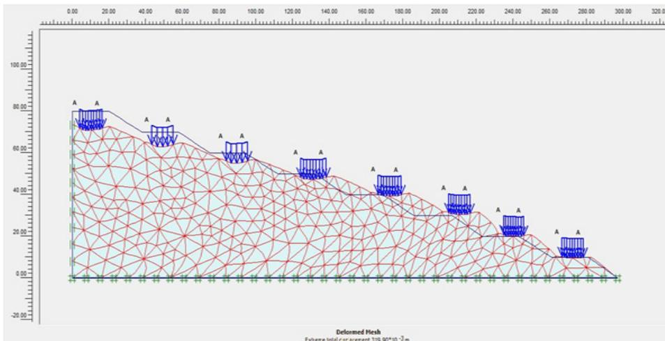
Figure 13. Deformed mesh.
