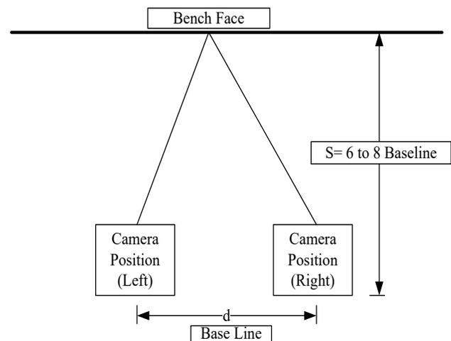
**Figure 3.** General layout for camera position<sup>10</sup>.
