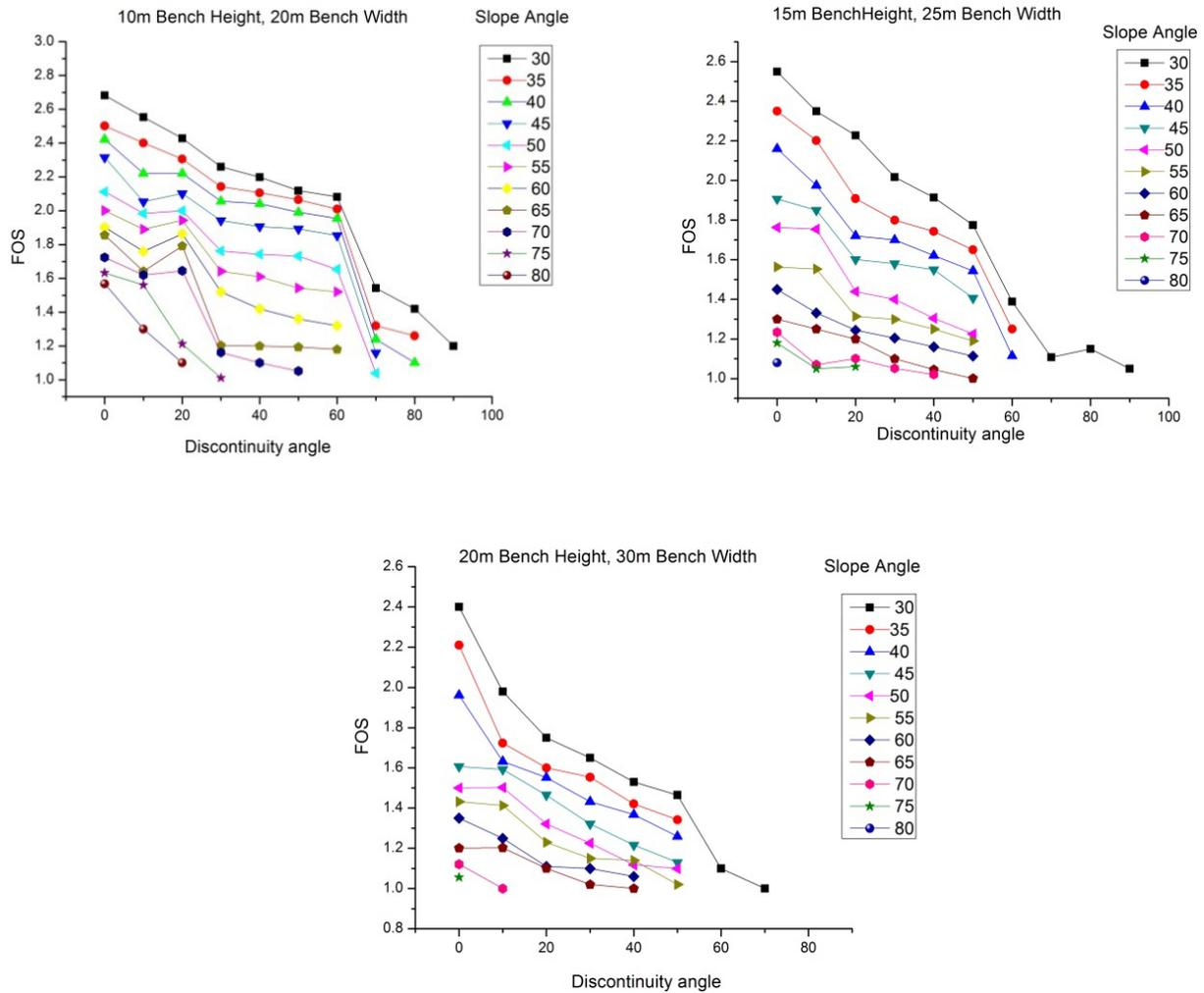
**Figure 19.** Influence of discontinuity angle on FOS for different slope angles.
