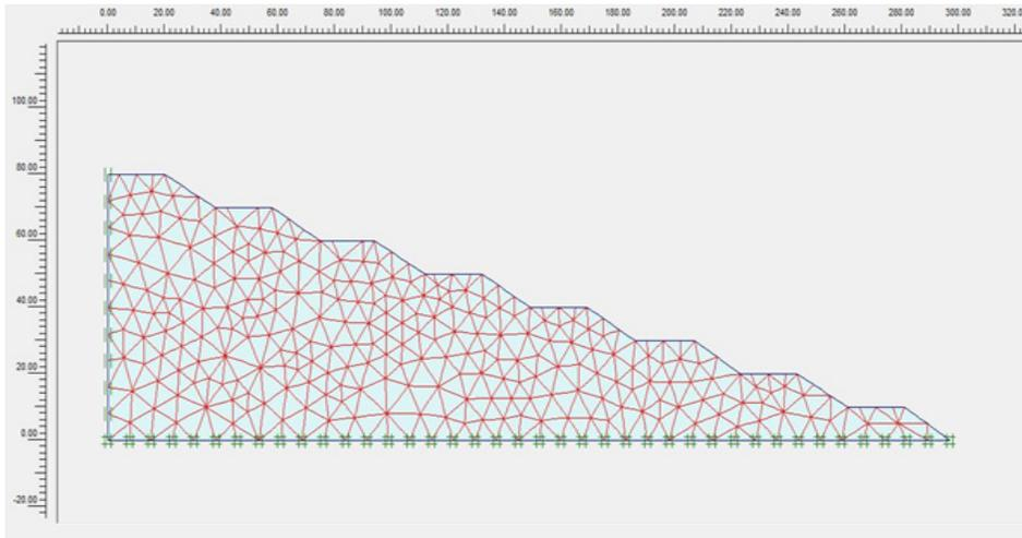
Figure 12. Mesh generated model.
