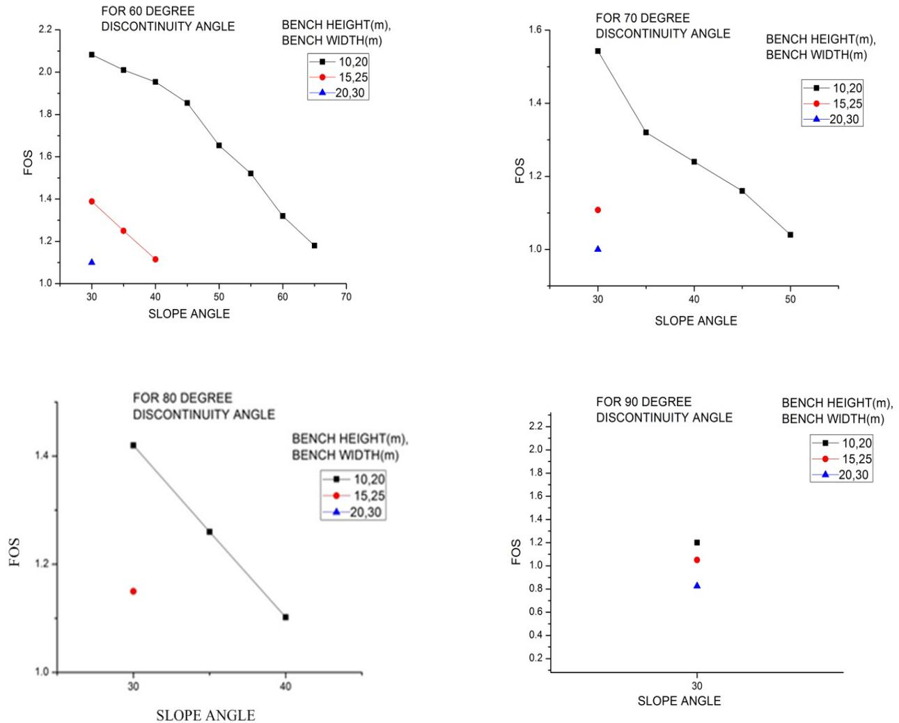
**Figure 17.** Influence of slope angle on FOS for different discontinuity angle and different bench height and bench width combination.
