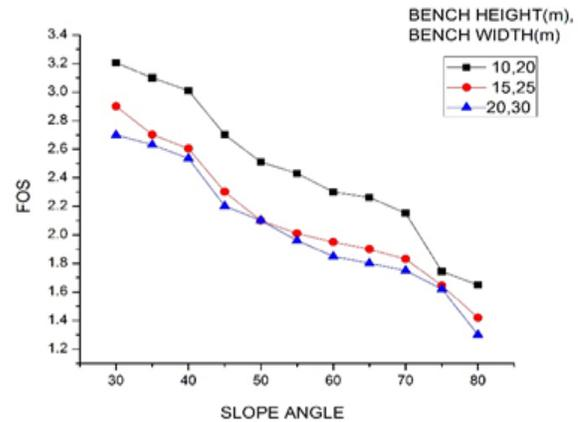
**Figure 16.** Influence of slope angle on FOS for different bench height and bench width combination.
