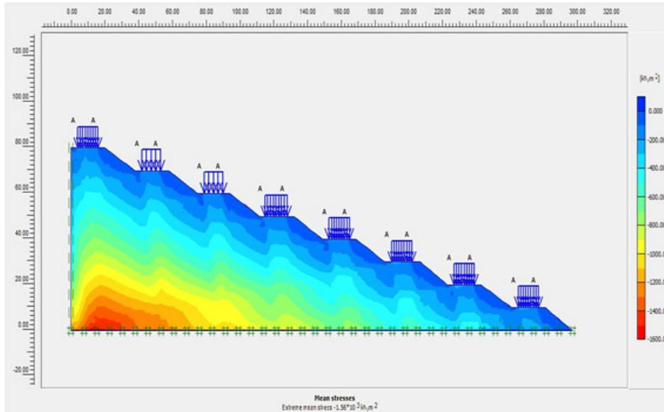
Figure 14. Effective stress developed in the model.
