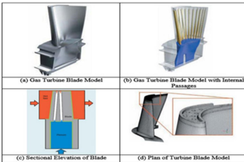
**Figure 2.** Segmental view and design gas turbine.
