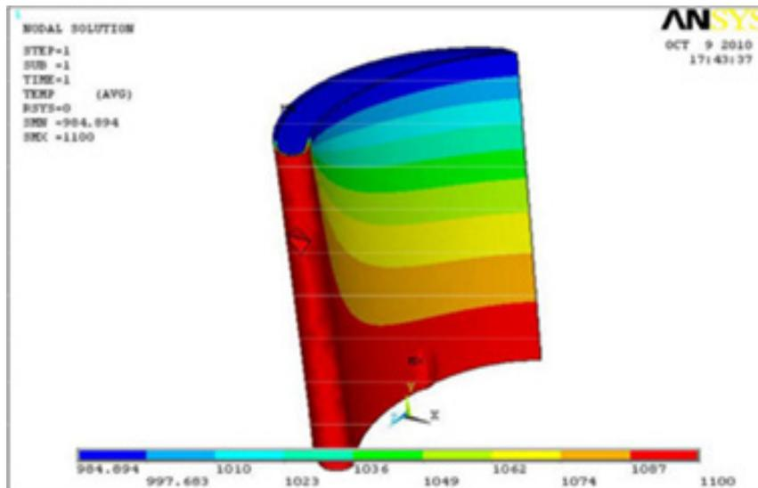
**Figure 19.** Temperature distribution analysis of turbine blade.
