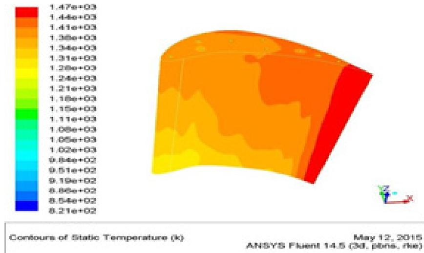
**Figure 9.** Contour of static temperature of 09 staggered holes.
