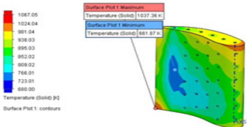
**Figure 15.** Representation of blade surface temperature on Pressure side of blade in staggered hole arrangement.
