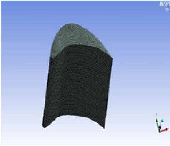
Figure 4. Meshing of blade.
