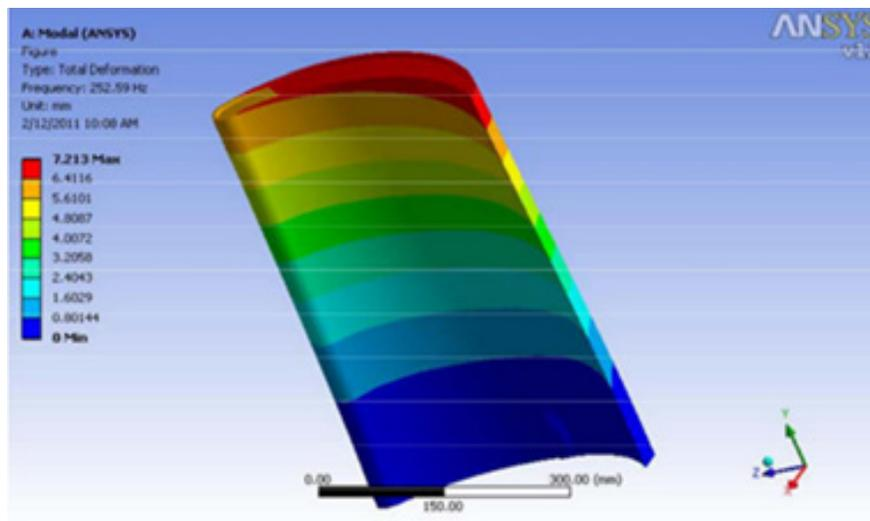
Figure 21. Vibration analysis of turbine blade with hole (frequency – 252.59 Hz).
