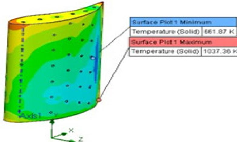
**Figure 16.** Representation of blade surface temperature on suction side of blade in staggered hole arrangement.
