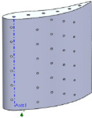
**Figure 1.** Geometry of staggered hole arrangement.
