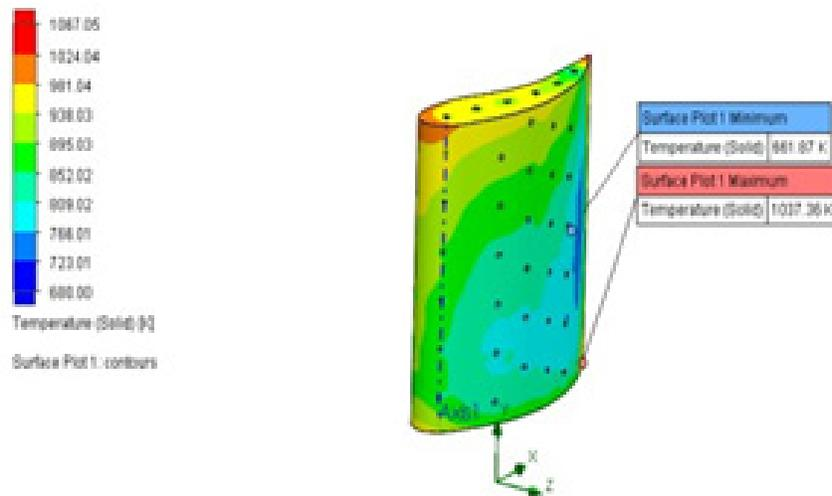
**Figure 17.** Representation of blade surface temperature on suction side of blade in inline hole arrangement
