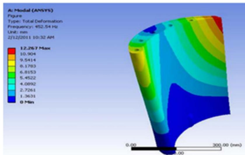
**Figure 20.** Vibration analysis of turbine blade without hole (frequency – 252.59 Hz).
