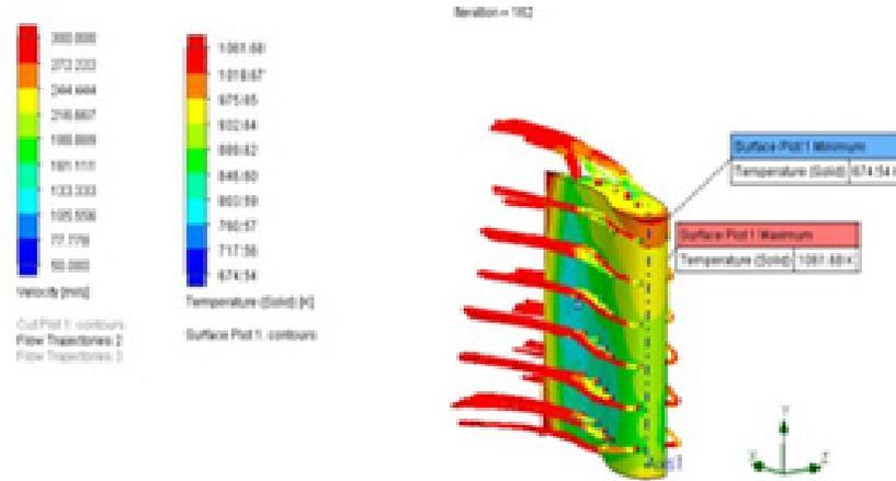
**Figure 13.** Representation of fluid flow Velocity on blade surface on pressure side in inline hole arrangement.
