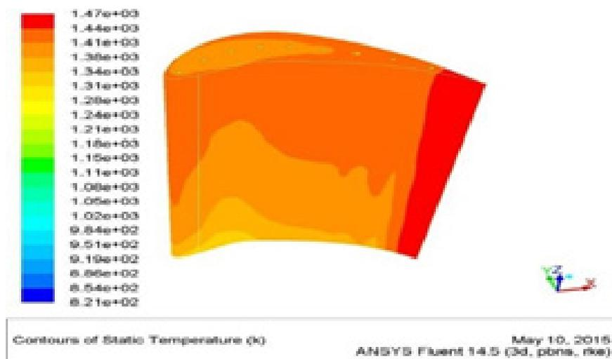
**Figure 8.** Counter Flow of static temperature 9 inline holes.
