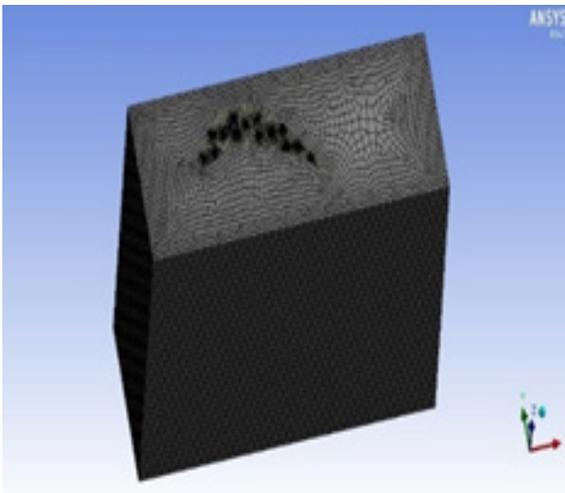
**Figure 7.** Meshing of 14 staggered holes.
