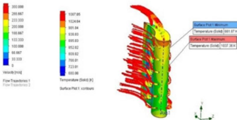
**Figure 14.** Representation of fluid flow Velocity on blade surface on pressure side in staggered hole arrangement.
