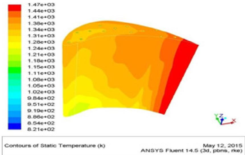
Figure 12. Contour of static temperature of 13 inline and staggered holes.
