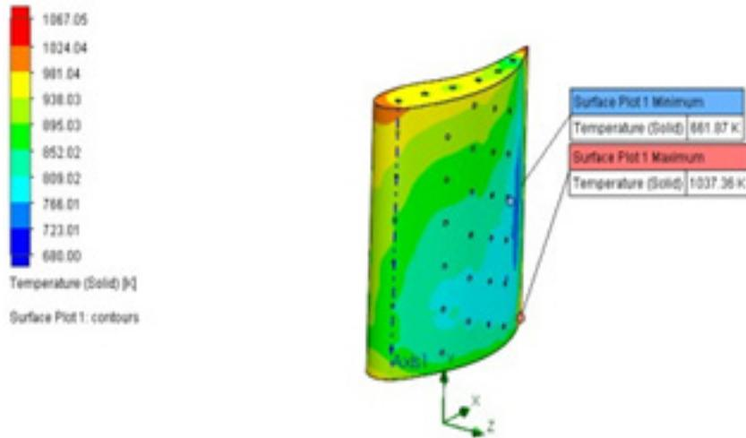
**Figure 18.** Representation of blade surface temperature on suction side of blade in staggered hole arrangement.
