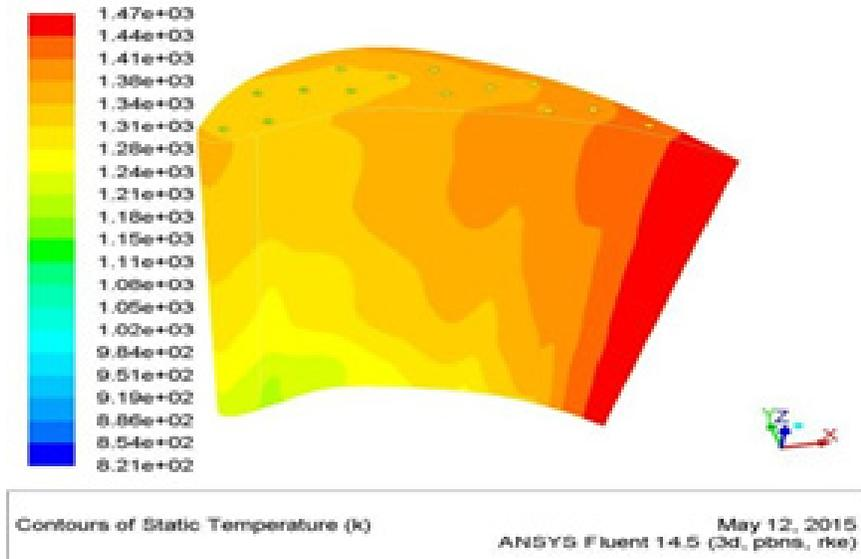
Figure 11. Contour of static temperature of 13 inline and staggered holes.
