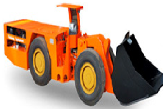
Figure 2. Diesel LHD used in underground metal mining.
