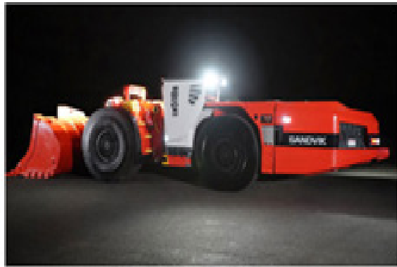
Figure 3. Battery LHD used in underground metal mining.
