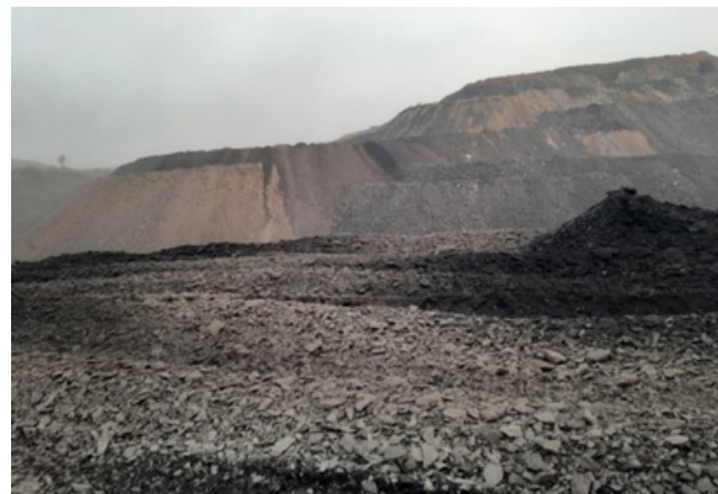
Figure 2. Coal and dirt bands/impurities cut by surface miners at Garjanbahal OCP.
