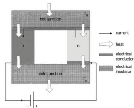
Figure 2. Thermoelectric couple schematic.
