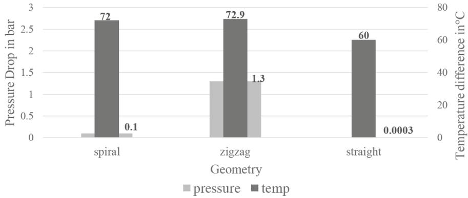
Figure 5.  $\Delta T$  and  $\Delta P$  vs flow geometry.
