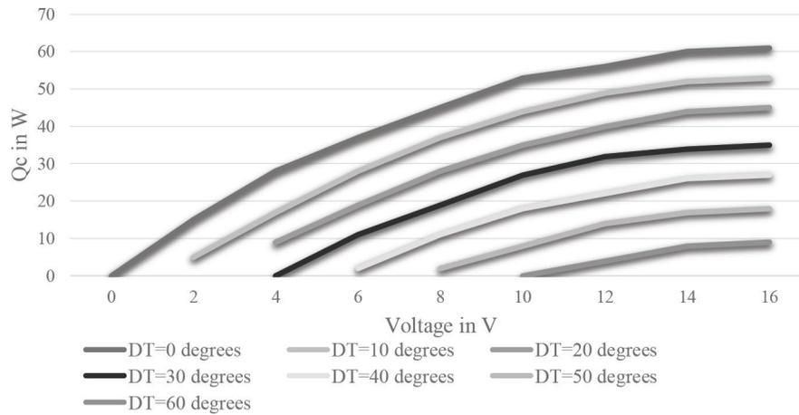
**Figure 9.** Standard performance graph  $V = f(\Delta T)$ . = 27°C (From Dymytrov, *et al*<sup>18</sup>).
