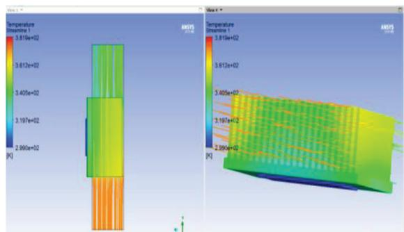
Figure 11. CFD Image in ANSYS Fluent for 21 CFM. Fluent Solver was used in finding the input and output heat from the pipe to calculate the heat absorbed by the fins.
