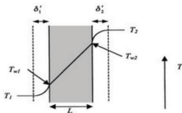
Figure 8. Conducting wall with convective heat transfer.
