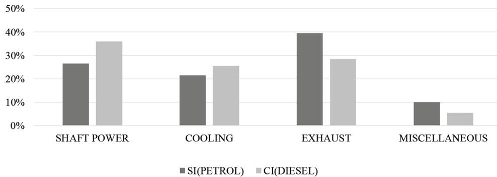
Figure 3. Waste energy in IC engines.
