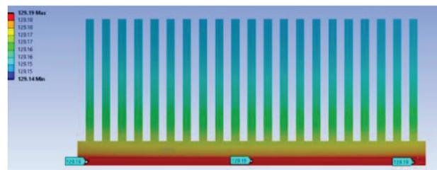
Figure 12. Steady-State analysis performed in ANSYS Workbench. The analysis is done to determine surface temperatures for different plate materials.
