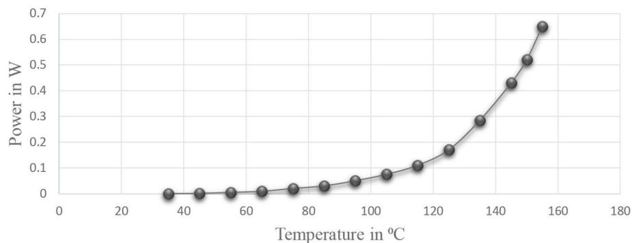
**Figure 1.** Variation of power output with temperature for thermoelectric generator.
