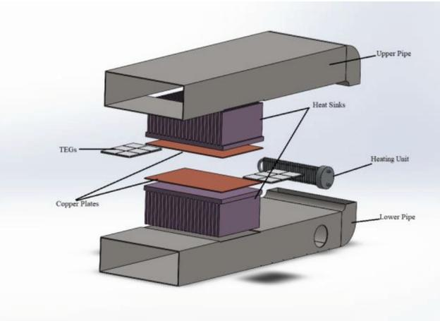
Figure 7. Exploded view of the proposed TEG model.
