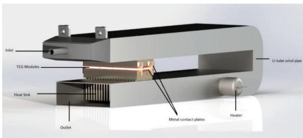
Figure 6. 3-D view of the proposed design of TEG.
