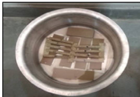
Figure 3. Cold water soaking test.
