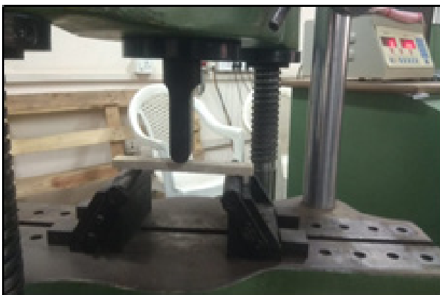
Figure 1. 3 Point bending test.
