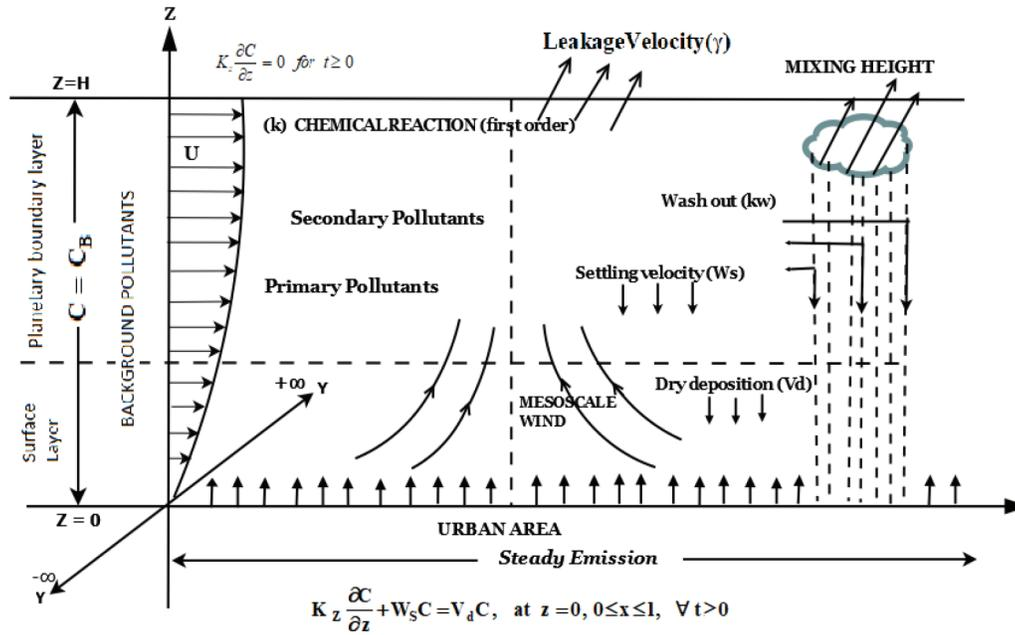
Figure 1. Physical layout of the model.
