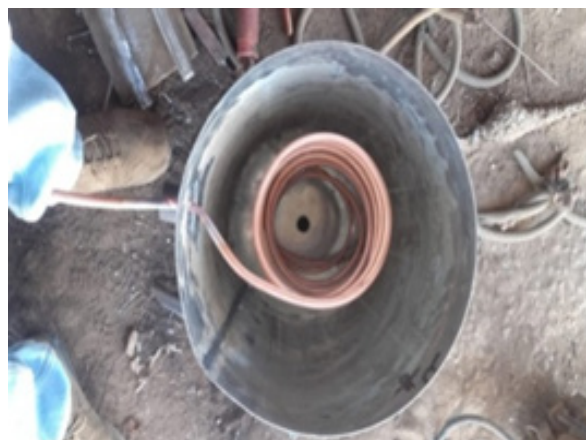
Figure 3. Fabricated pre-heating chamber.
