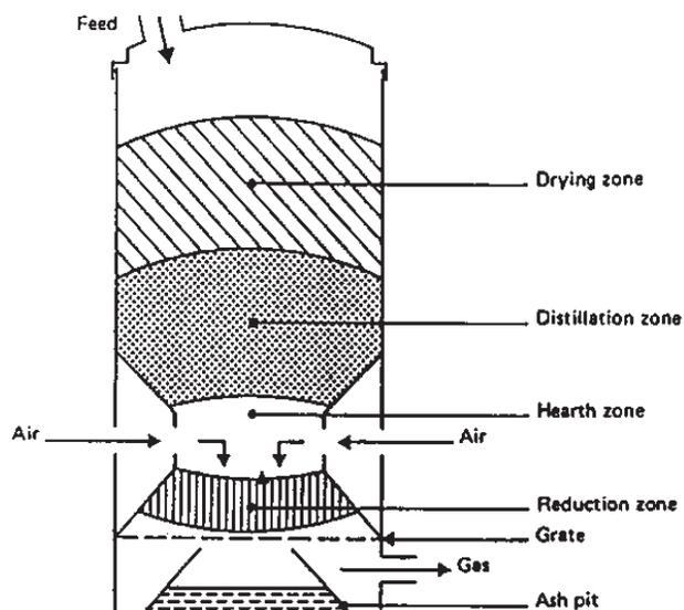
Figure 2. Downdraft Gasifier.
