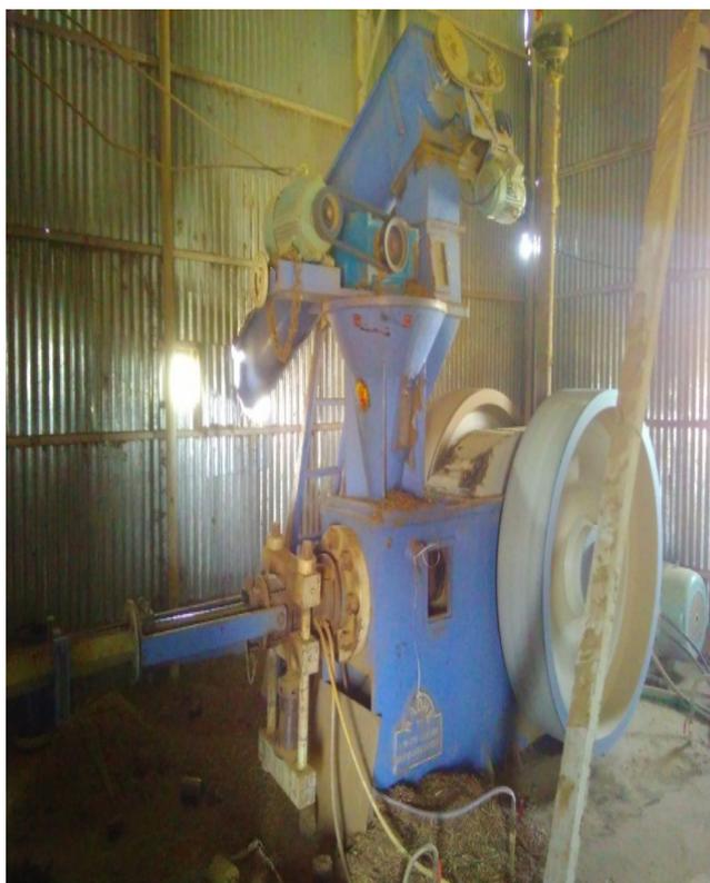
**Figure 5.** Compressed type Briquetting plant.
