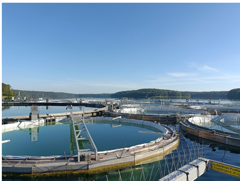
A look into the sea laboratory for water ecology and inland fishing (IGB) in an experimental cylinder with clear water back left one with brown coloured water.
