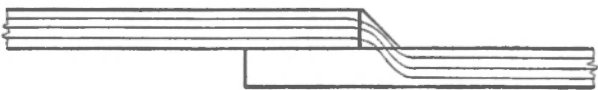
(b) Example of lap weld having a more even distribution of stress through weld.
