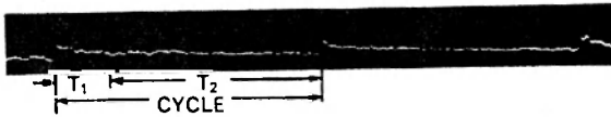
Fig. 5. Oscillograph of a typical Arc Voltage transient in free flight mode of metal transfer.
