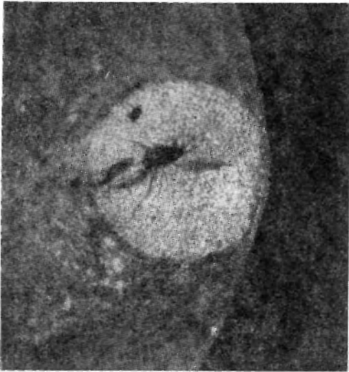
Fig. 1. Photograph of a "white spot" (fish eye) on a broken tensile test specimen of weld metal produced by arc welding. R. Castro-1937-author's archives.
