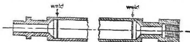
Fig. 19. Feed tubes for rock drilling made by friction welding of male and female threaded coupling ends to standard lengths of tube. The tubes are usually 64 to 82 mm dia. and about 3 mm long.
