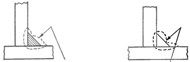
Fig. 3. Profile of typical uneconomic fillet welds.
