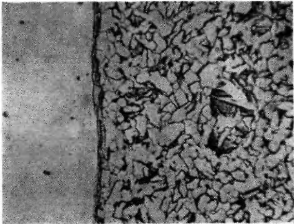
Fig.—4b (Microphoto shows the complete bonding of mild steel to stainless steel. Unetched portion is stainless steel side, etched portion is mild steel).
