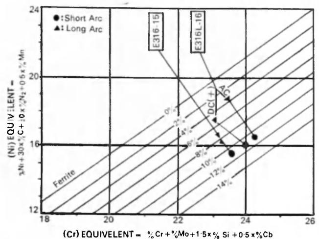
Fig 4. Effect of Arc length on Ferrite Content (Ref. 5)
