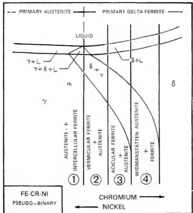
Fig 3 Schematic Pseudo-Binary Diagram of the Fe-Cr-Ni Ternary System (Ref. 1)
