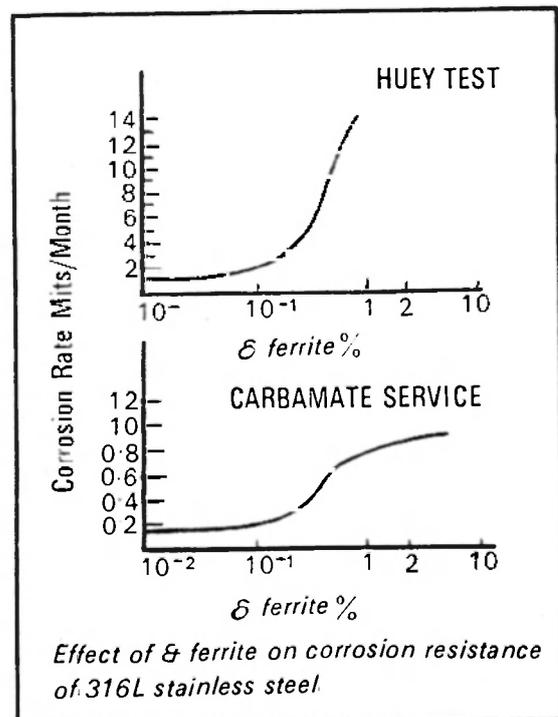
Fig. 5 Corrosion rates in urea Service.
