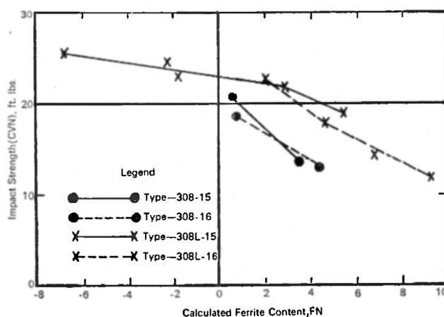
Fig. 6—Impact strength (vs) Ferrite Content for 308/308L grades tested at -196°C (Ref. 18).
