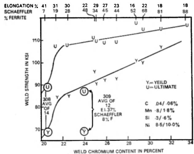
Fig 0—Effect of Ferrite on Tensile Properties (Ref. 7)
