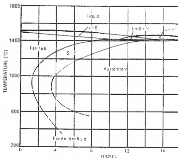
Fig 1 Vertical Section of very low carbon Fe-Cr-Ni Alloys at 18% Cr. (Ref. 20)
