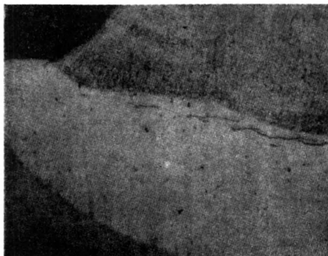
Heat affected zone hydrogen cracking—a common consequence of incorrect preheating practice.
