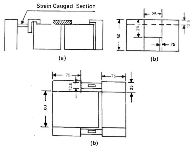
G-BOP test to measure stress &amp; restraint
