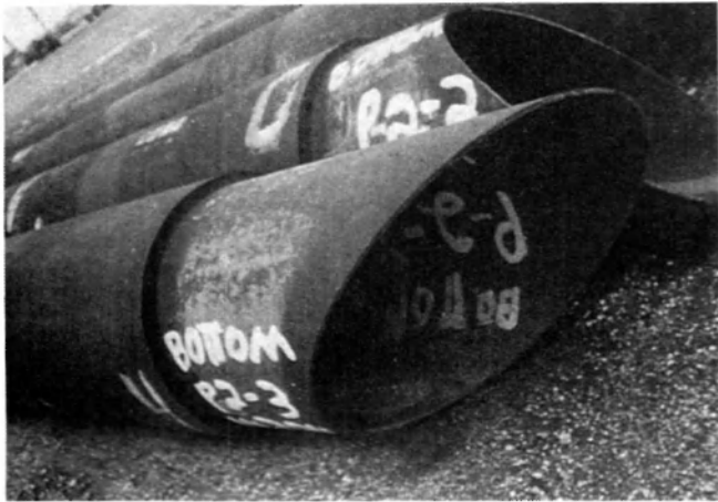
Fig. 5. Examples of "stabbing points" for horizontal or vertical applications
