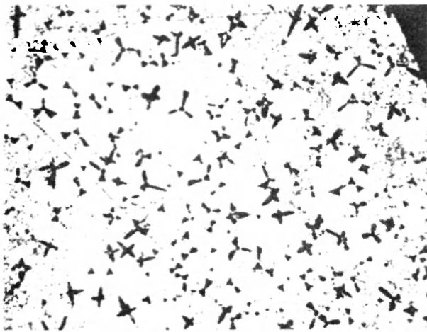
Fig.23. Micrograph of metallic crystal (brazing tip used), (X600)
