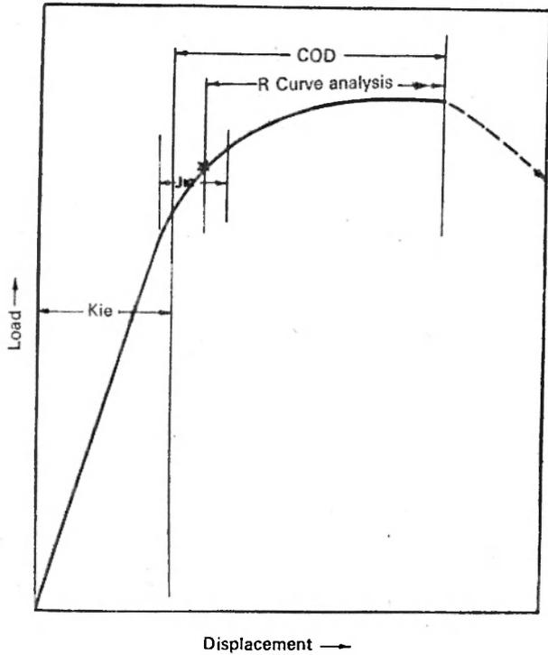
Fig. 1: Valid ranges of fracture mechanics concepts
