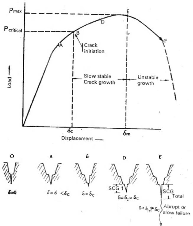
Fig. 2: Crack opening displacement—principle
