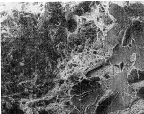
(a) Stretch zone/cleavage fracture  $\times 650$
