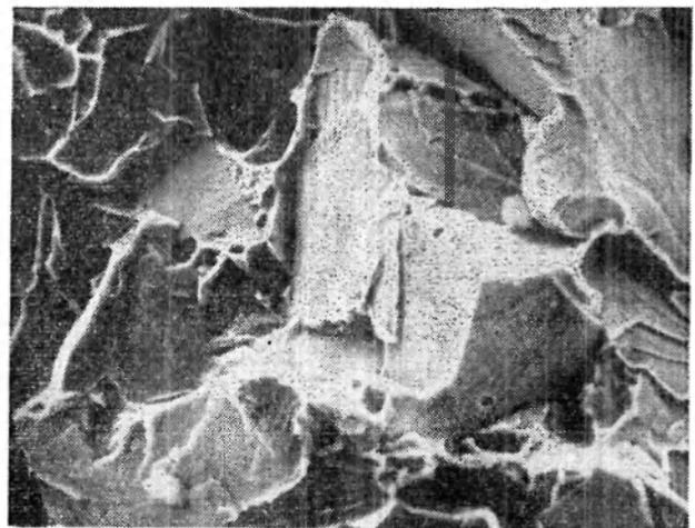
(b) Cleavage fracture
