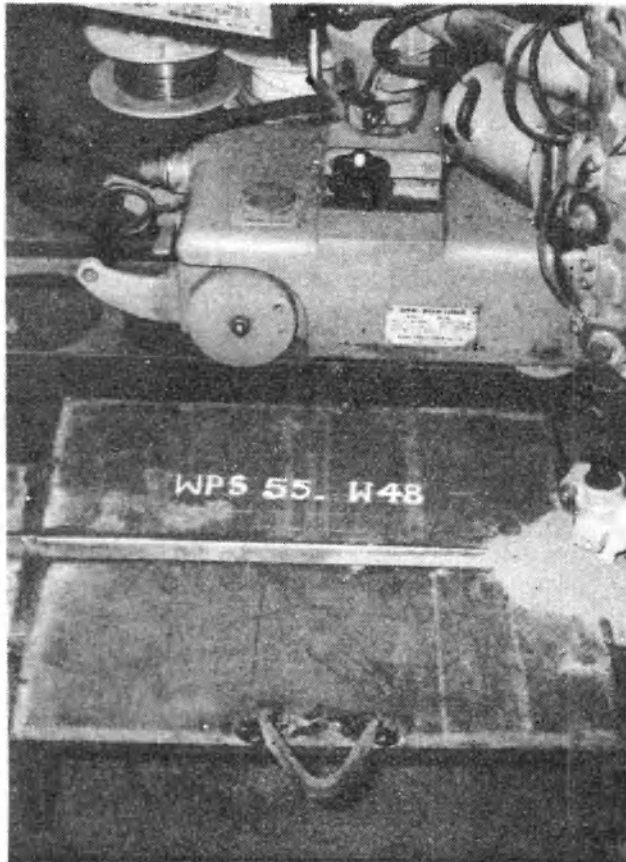
Fig. 8 Arrangement for submerged ARC one side FAB Welding (view from top).
