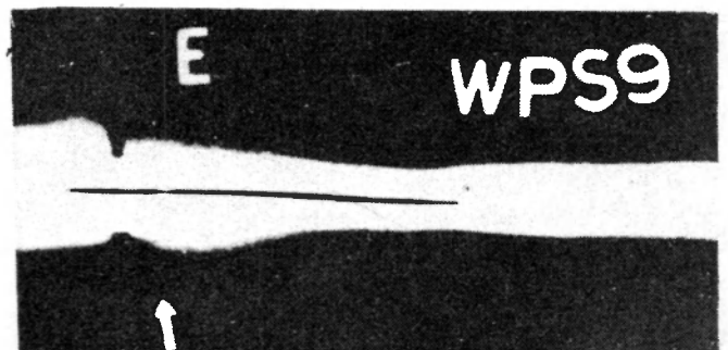
Fig. 4 Radiograph showing end crack in one side FCB Welding.
