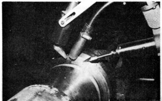
Fig. 8 : CONFIGURATION OF WELDING TORCH SEAM TRACKER AND ARC OSCILLATOR PROBES
