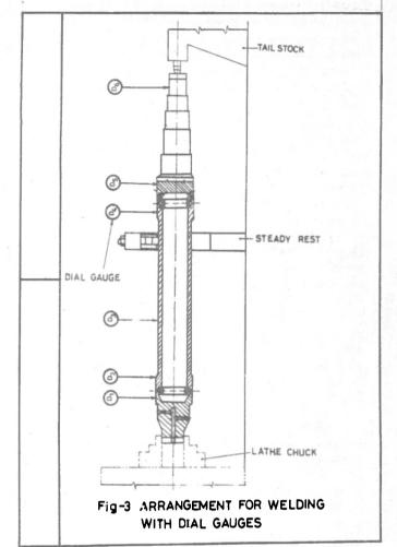
the tail stock centre was removed and shielding gas flow on the root side was stopped. After completion of welding both the joints were liquid penetrant tested and were found to<sup>4</sup> be defect free.
