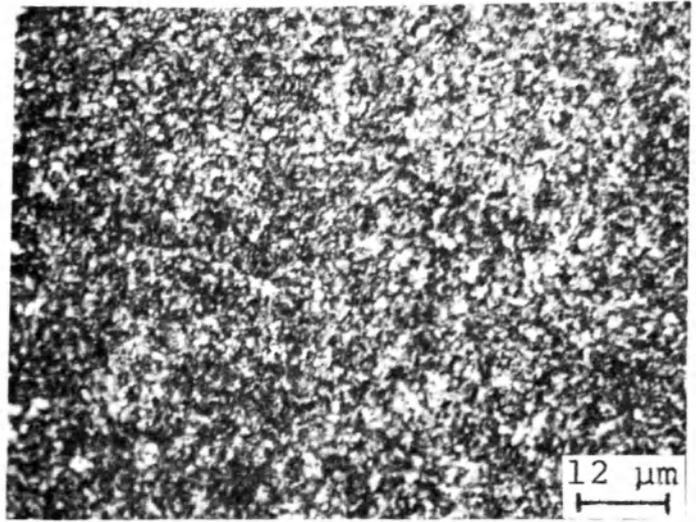
Fig. 2 Microstructure of the fine grain region of HAZ.
