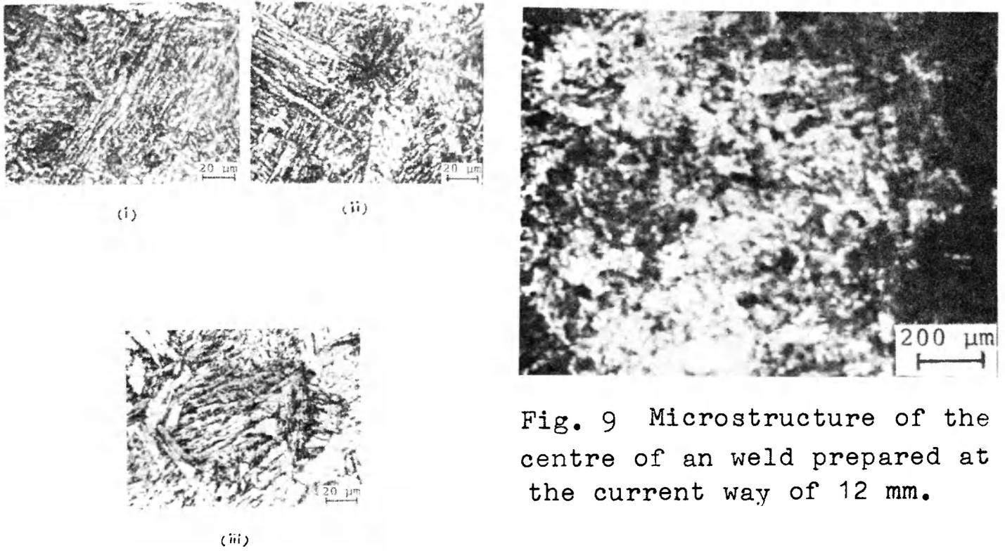
Fig. 9 Microstructure of the centre of an weld prepared at the current way of 12 mm.
