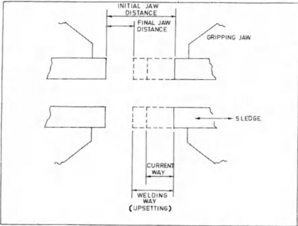
Fig. 1 Schematic diagram of the welding process.
