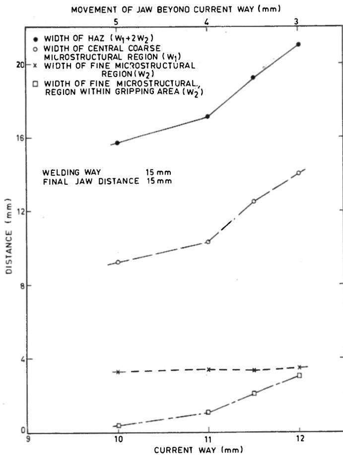
Fig. 4 Effect of current way on the width of different microstructural region in HAZ.
