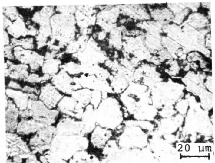
Fig. 7 Microstructure of base metal.
