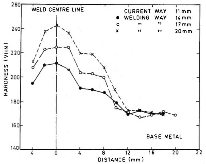
Fig.12 Effect of welding way on the hardness behaviour across the weld.
