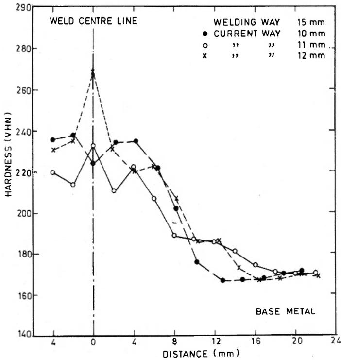
Fig.11 Effect of current way on the hardness behaviour across the weld.
