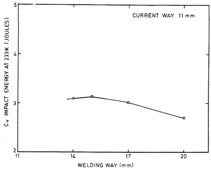
Fig.14 Effect of welding way on the C<sub>v</sub> impact value of the weld centre.
