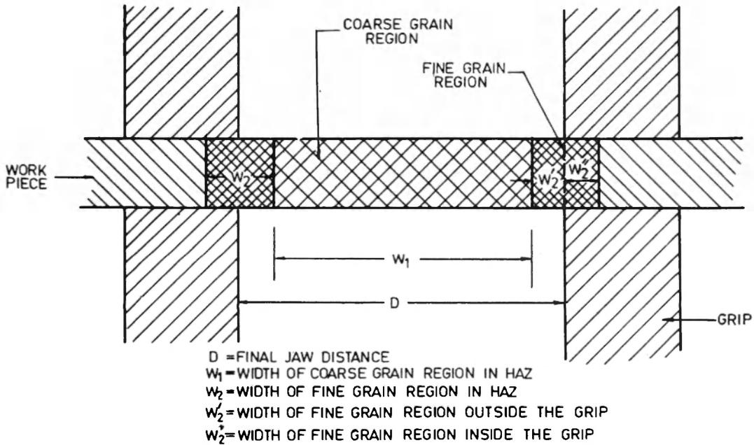
Fig. 3 Schematic diagram of the location of different microstructural region in HAZ.
