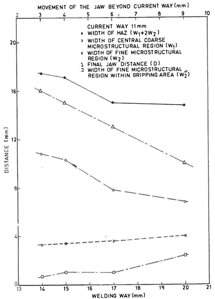
Fig. 5 Effect of welding way on the width of different microstructural region in HAZ.
