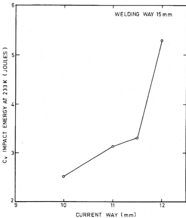
Fig.13 Effect of current way on the C<sub>v</sub> impact value of the weld centre.
