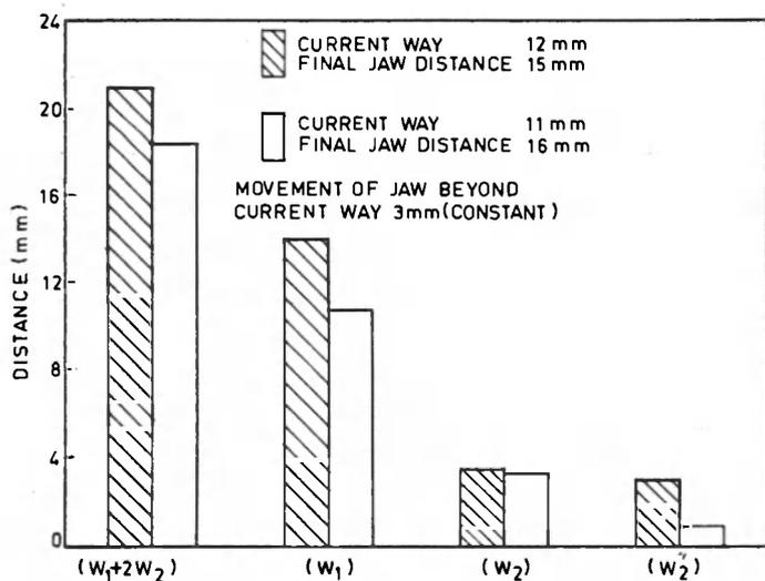
Fig. 6 At a given movement of Jaw beyond the current way the effect of current way on the width of different microstructural region in HAZ.
